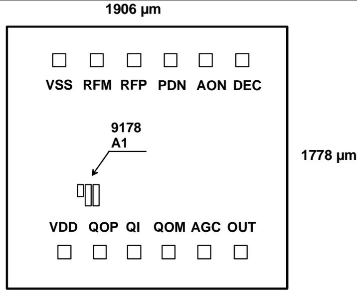
DIE size = 1.91 x 1.78 mm; PAD size = 100 x 100 µm except for VSS PAD size 104 x 112 µm
