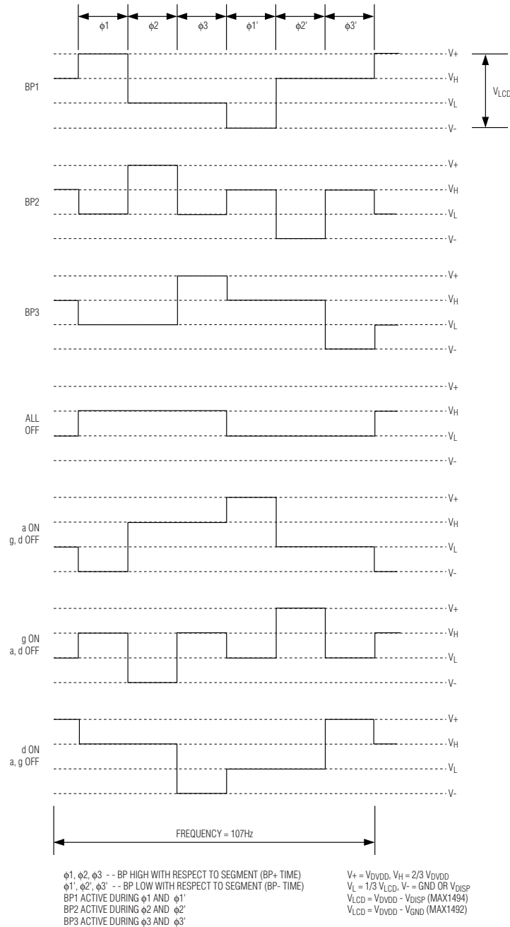
Figure 9. LCD Voltage Waveform—Combinations 1–4 (BP-, SEG2/5/8)
