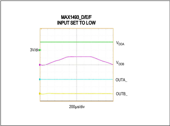
Figure 5. Undervoltage Lockout Behavior (MAX1493_D/E/F Low)
