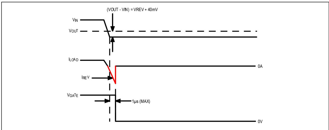
Figure 3. Reverse-Voltage Fault
