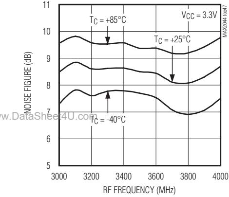
**NOISE FIGURE vs. RF FREQUENCY**
