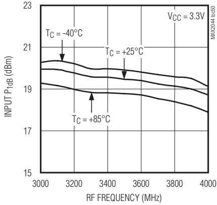
**INPUT P<sub>1dB</sub> vs. RF FREQUENCY**
