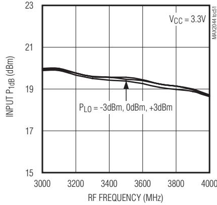
**INPUT P<sub>1dB</sub> vs. RF FREQUENCY**
