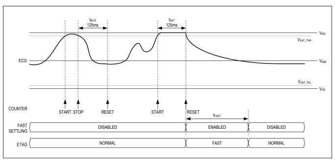
Figure 6. Automatic Fast Settling Behavior
