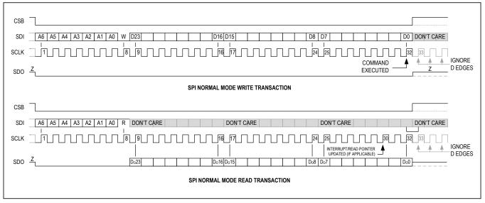
Figure 8. SPI Normal Mode Transaction Diagrams
