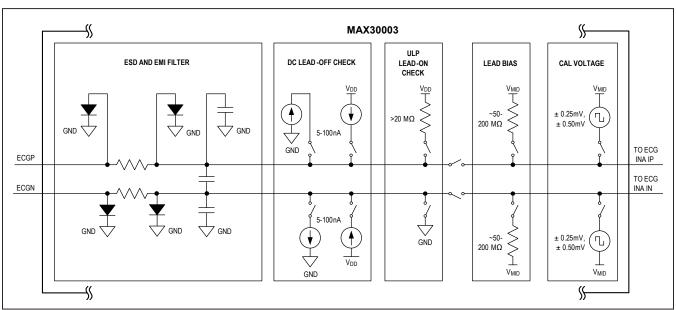
Figure 3. ECG Input MUX
