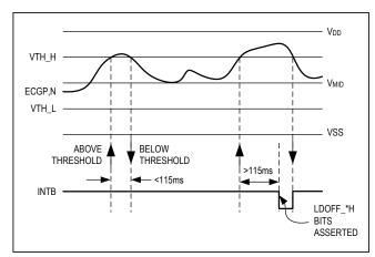
Figure 4. Lead-Off Detect Behavior
