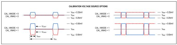
Figure 10. Calibration Voltage Source Options
