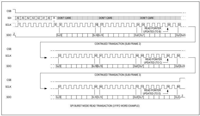
Figure 9. SPI Burst Mode Read Transactions Diagrams
