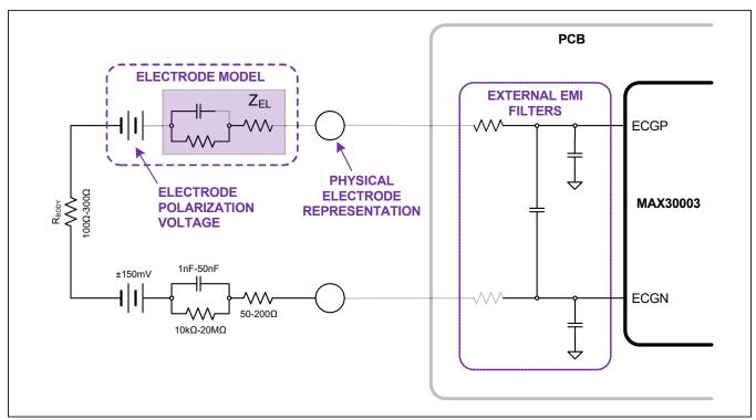
Figure 12. Two Electrode Heart Rate Monitoring for Fitness
