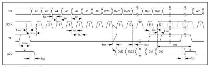
Figure 1a. SPI Timing Diagram
