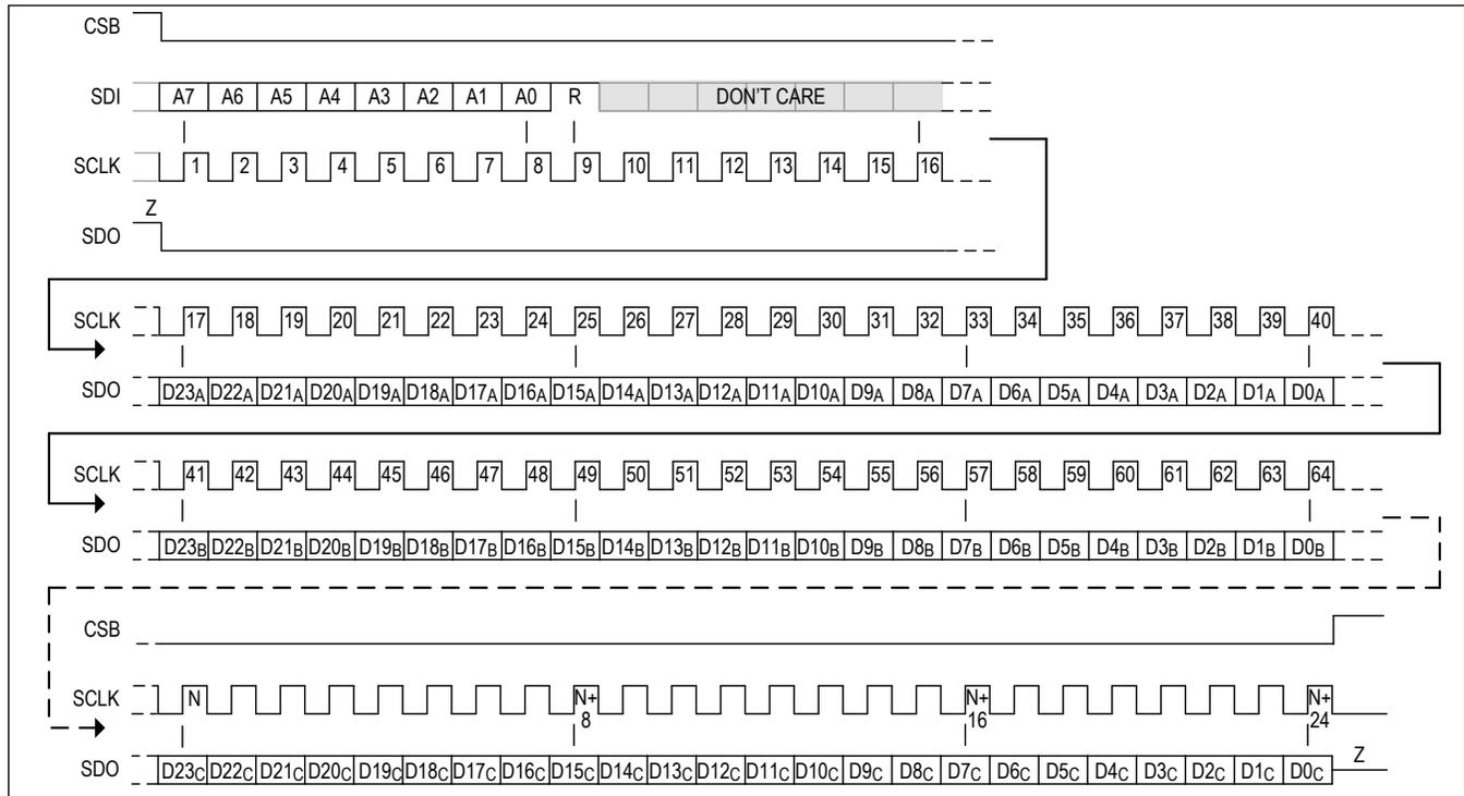
Figure 20. SPI FIFO Burst Mode Read Transaction
