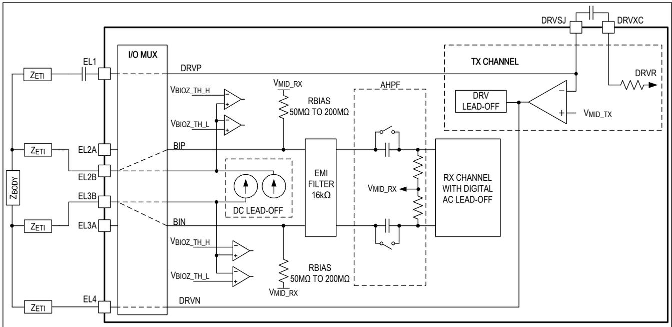
Figure 14. BioZ DC Lead-Off Detection with Internal Sense
