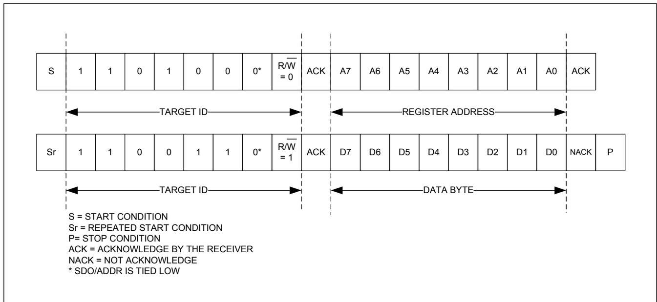
Figure 26. I<sup>2</sup>C Single-Byte Read Transaction
