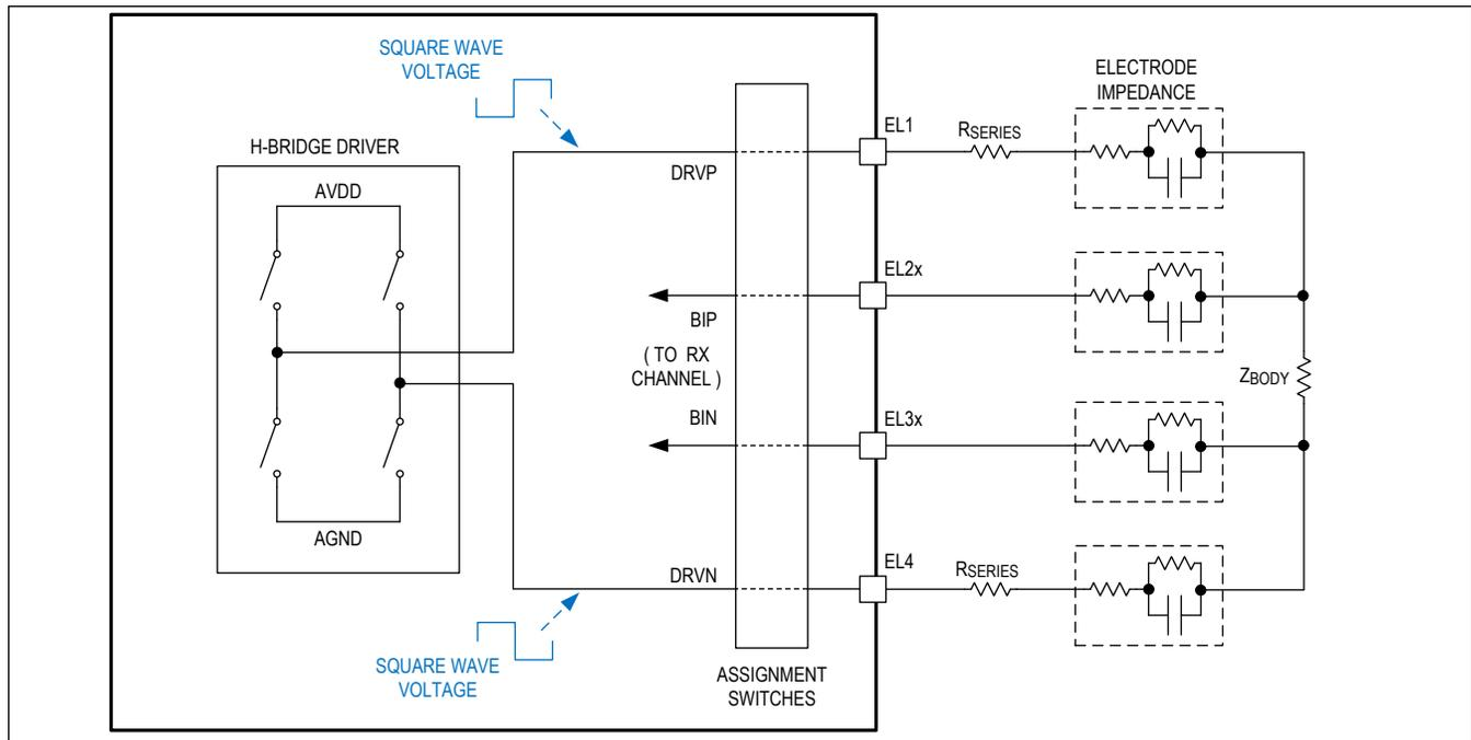
Figure 8. Bioimpedance Stimulus Generator — H-Bridge Square-Wave Voltage Mode
