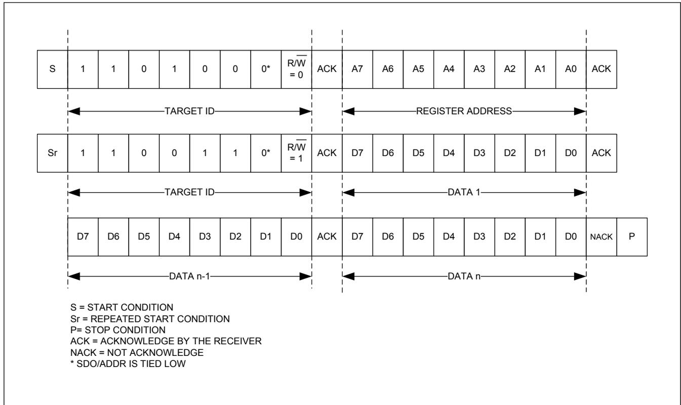
Figure 27. I<sup>2</sup>C Multibyte Read Transaction
