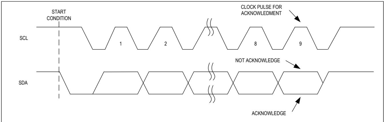
Figure 23. I<sup>2</sup>C Acknowledge Bit
