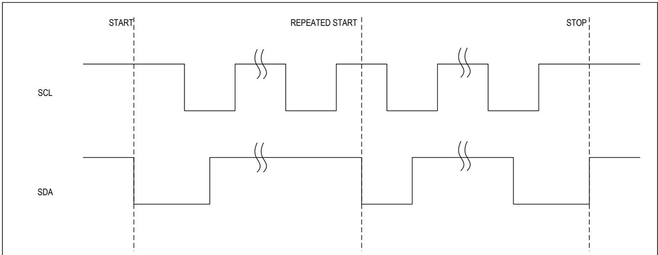
Figure 22. I<sup>2</sup>C START, STOP, and REPEATED START Conditions
