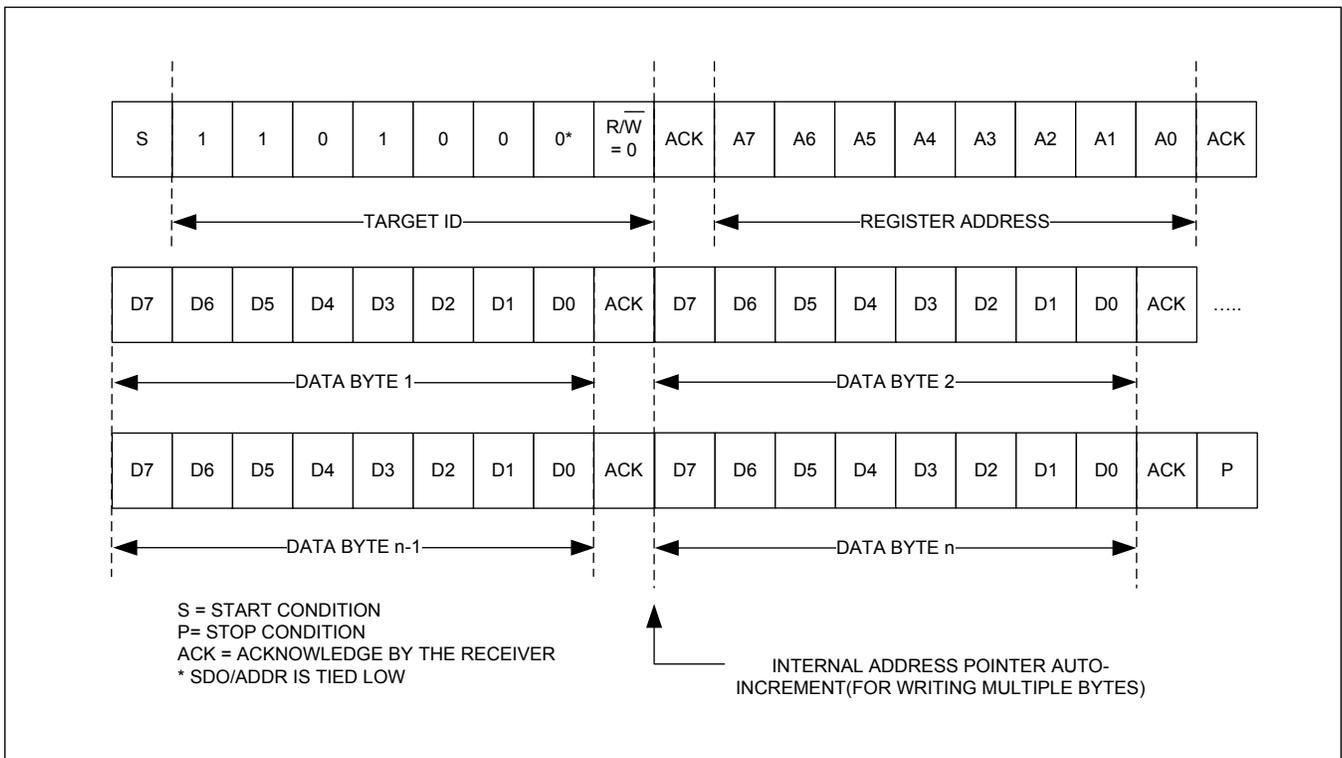
Figure 25. I<sup>2</sup>C Multibyte Write Transaction
