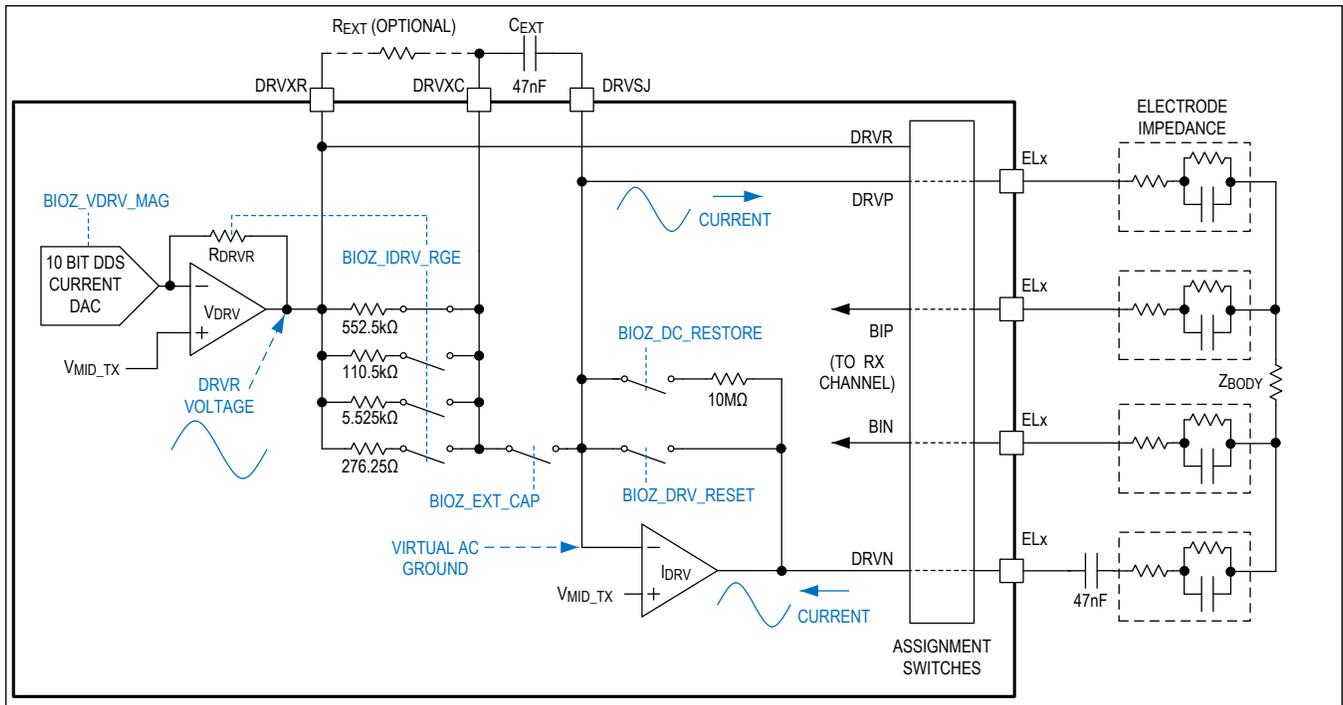
Figure 6. Bioimpedance Stimulus Generator — Sine-Wave Current Mode
