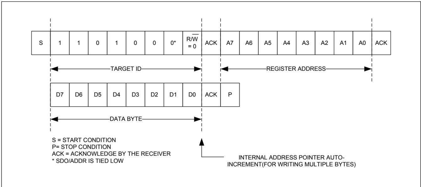
Figure 24. I<sup>2</sup>C Single-Byte Write Transaction
