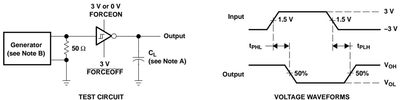
NOTES: A.  $C_L$  includes probe and jig capacitance.
