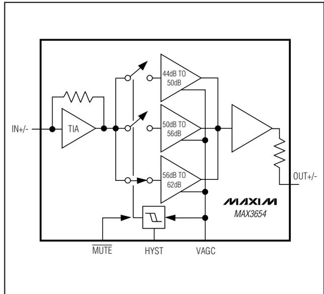
Figure 3. Functional Diagram
