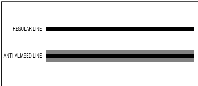
Figure 9. Anti-Aliased Line Drawing
