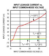
$(V_{CM} = V_{RS+} = V_{RS-} = +50V, V_{DD} = +3.3V, V_{SENSE} = V_{RS+} - V_{RS-} = 0V, V_{REF1} = V_{DD}/2, V_{REF2} = V_{DD}/2, G = 20V/V, T_A = +25^{\circ}C, unless otherwise noted.)$
