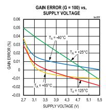
$(V_{CM} = V_{RS+} = V_{RS-} = +50V, V_{DD} = +3.3V, V_{SENSE} = V_{RS+} - V_{RS-} = 0V, V_{REF1} = V_{DD}/2, V_{REF2} = V_{DD}/2, G = 20V/V, T_A = +25^{\circ}C, unless otherwise noted.)$
