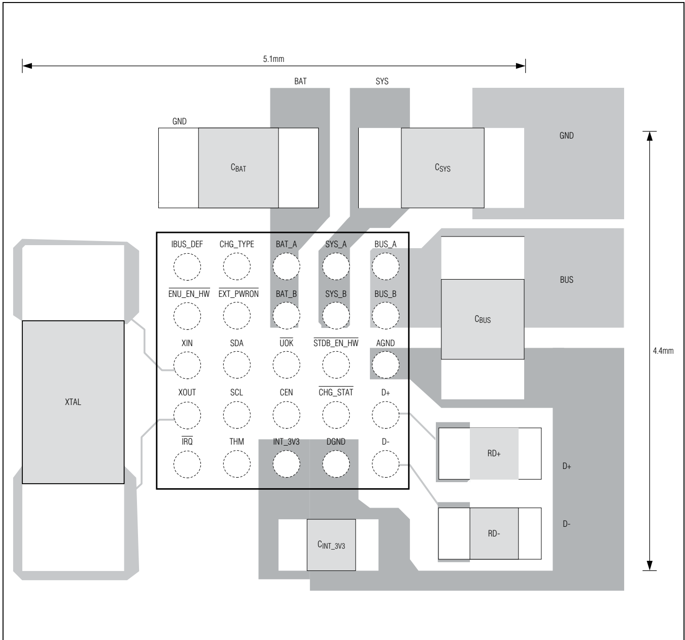
Figure 25. Recommended PCB Layout for Full Speed
