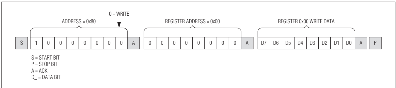
Figure 28. Format for I 2 C Write
