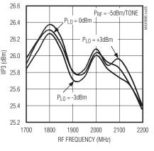
**INPUT IP3 vs. RF FREQUENCY**
