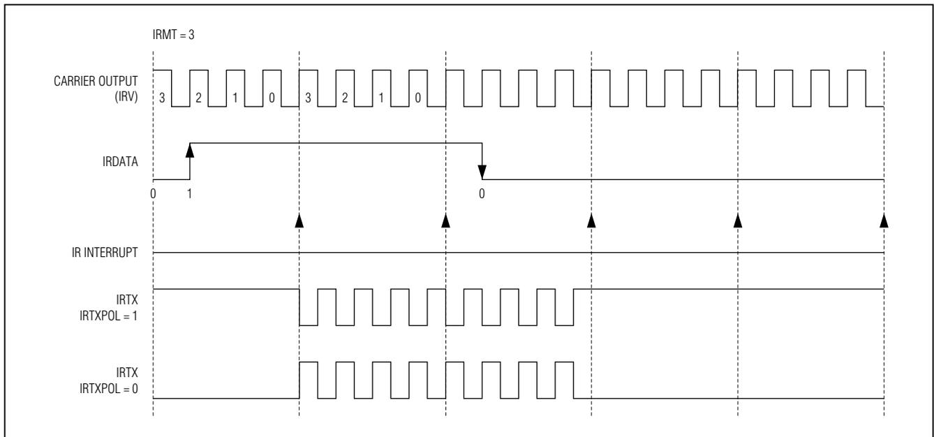
Figure 3. IR Transmission Waveform (IRCFME = 0)
