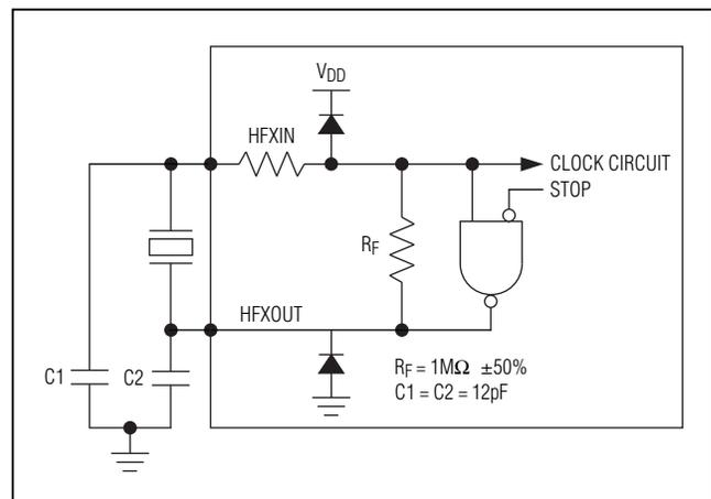
Figure 9. On-Chip Oscillator
