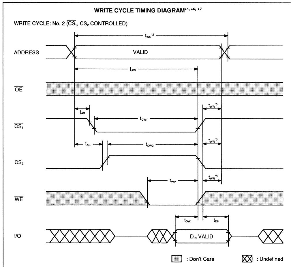
**Note:** \*1 If  $\overline{CS}$  goes high simultaneously with  $\overline{WE}$  high, the output remains in high impedance state.
