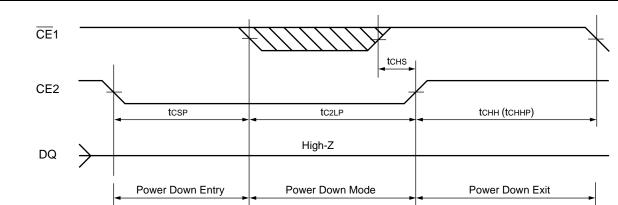
Note: This Power Down mode can be also used as a reset timing if "Power-up timing" above could not be satisfied and Power Down program was not performed prior to this reset.
