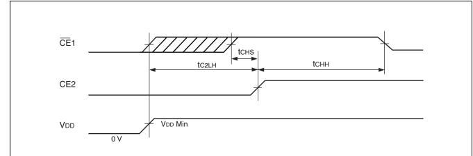
Note : The  $t_{\text{C2LH}}$  specifies after  $V_{\text{DD}}$  reaches specified minimum level.
