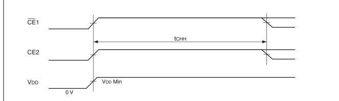
Note: The tchh specifies after Vdd reaches specified minimum level and applicable to both  $\overline{\text{CE}}1$  and CE2. If transition time of Vdd (from 0 V to Vdd Min) is longer than 50 ms, Power-up Timing #1 must be applied.
