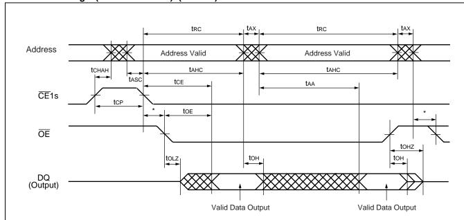
Note: CE2s and  $\overline{\text{WE}}$  must be HIGH for entire read cycle.
