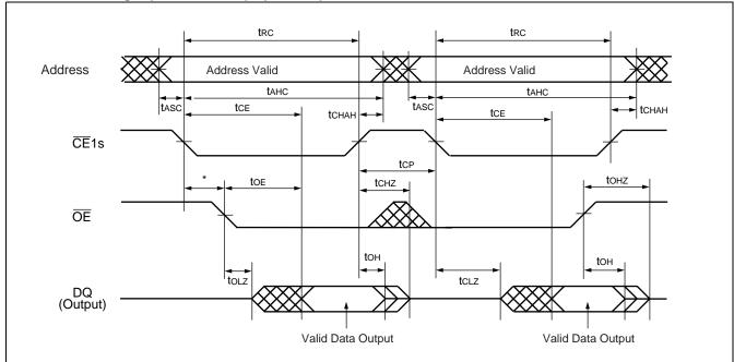
Note : CE2s and  $\overline{\text{WE}}$  must be HIGH for entire read cycle.
