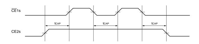
Note: tcap is not applicable CE2s HIGH pulse width while  $\overline{\text{CE}}1\text{s}$  stays LOW and CE2s should not use as a read and write timing control signal in stead of  $\overline{\text{CE}}1\text{s}$ .
