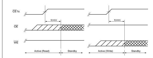
Note: Both  $t_{CHOX}$  and  $t_{CHWX}$  define the earliest entry timing for Standby mode. If either of timing is not satisfied, it takes  $t_{RC}$  (min) period from either last address transition or  $\overline{CE}1s$  Low to High transition.
