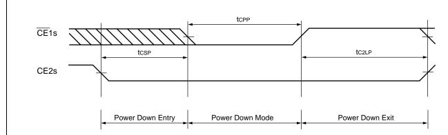
Note: A minimum of two dummy read cycle must be performed prior to regular read and write operation after tc2LR Otherwise  $\overline{\text{CE}}$ 1s must kept High for tc1HP period after tc2LR
