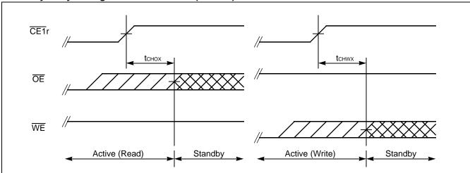
Note: Both tchox and tchwx define the earliest entry timing for Standby mode. If either of timing is not satisfied, it takes trace (Min) period from either last address transition of A<sub>0</sub> and A<sub>1</sub>, or  $\overline{CE1}$ r Low to High transition.
