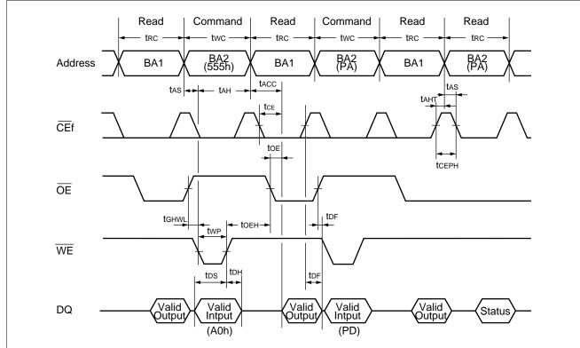
Note: This is example of Read for Bank 1 and Embedded Algorithm (program) for Bank 2.
