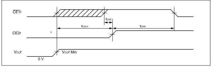
\*: It is recommended CE2r to kept at Low during Vccr power-up. The tc2LH specifies after Vccr reaches specified minimum level.
