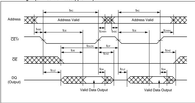
Note : CE2r and  $\overline{\text{WE}}$  must be High for entire read cycle.
