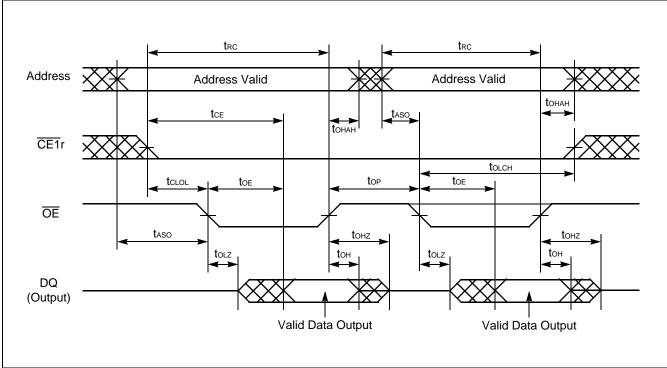
Note : CE2r and  $\overline{\text{WE}}$  must be High for entire read cycle.
