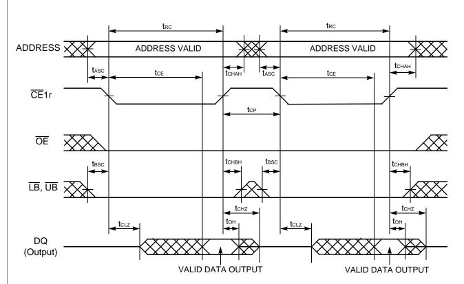
Note: CE2r and  $\overline{\text{WE}}$  must be High for entire read cycle. Either or both  $\overline{\text{LB}}$  and  $\overline{\text{UB}}$  must be Low when both  $\overline{\text{CE}}$ 1r and  $\overline{\text{OE}}$  are Low.
