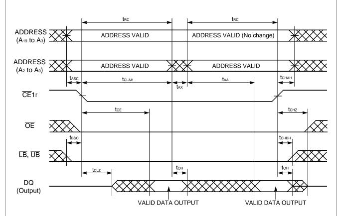
Note : CE2r and  $\overline{\text{WE}}$  must be High for entire read cycle.
