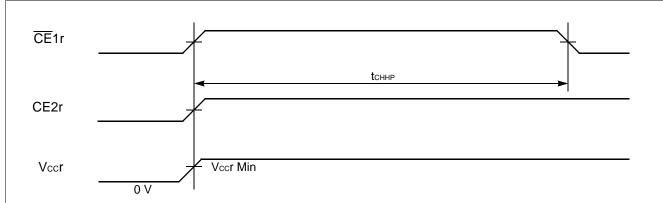
Note: Both  $\overline{\text{CE}}1\text{r}$  and  $\overline{\text{CE}}2\text{r}$  must be High together with Vccr. Otherwise either POWER-UP Timing #1 or #2 must be used for proper operation.
