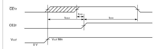
Note: The tc2LH specifies after Vccr reaches specified minimum level.
