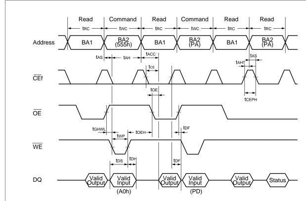
Note: This is example of Read for Bank 1 and Embedded Algorithm (program) for Bank 2.
