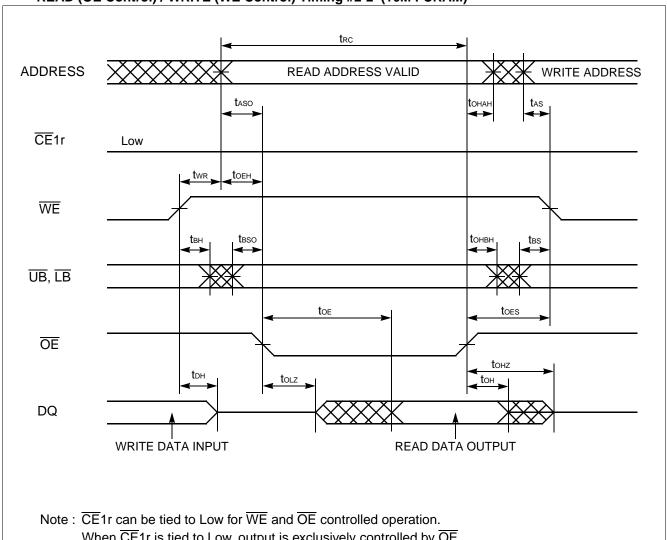
When  $\overline{\text{CE}}1\text{r}$  is tied to Low, output is exclusively controlled by  $\overline{\text{OE}}$ .
