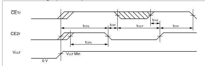
Note: The tc2HL specifies from CE2r Low to High transition after Vccr reaches specified minimum level.
