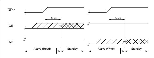
Note: Both tchox and tchwx define the earliest entry timing for Standby mode. If either of timing is not satisfied, it takes trc(Min) period from either last address transition of A<sub>0</sub>, A<sub>1</sub> and A<sub>2</sub>, or  $\overline{\text{CE}}$ 1r Low to High transition.
