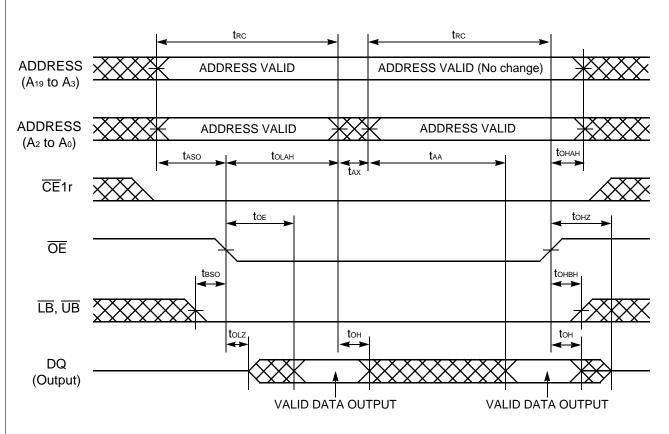
Note : CE2r and  $\overline{\text{WE}}$  must be High for entire read cycle. Either or both  $\overline{\text{LB}}$  and  $\overline{\text{UB}}$  must be Low when both  $\overline{\text{CE}}$ 1r and  $\overline{\text{OE}}$  are Low.
