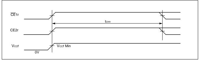
Note: The tchh specifies after Vccr reaches specified minimum level and applicable both  $\overline{\text{CE}}1\text{r}$  and CE2r.
