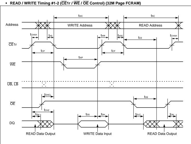
Note :  $\overline{OE}$  can be Low fixed in write operation under  $\overline{CE1r}$  control  $\overline{RD}$ - $\overline{WR}$ - $\overline{RD}$  operation.
