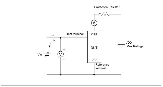
Note : The voltage V<sub>IN</sub> is increased gradually and the current I<sub>IN</sub> of 300 mA at maximum shall flow. Confirm the latch up does not occur under I<sub>IN</sub> = ± 300 mA. In case the specific requirement is specified for I/O and I<sub>IN</sub> cannot be 300 mA, the voltage shall be
