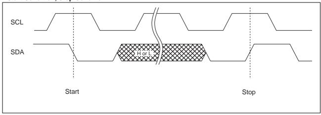
Note: At the write operation, the FRAM device does not need the programming wait time (twc) after issuing the Stop Condition.
