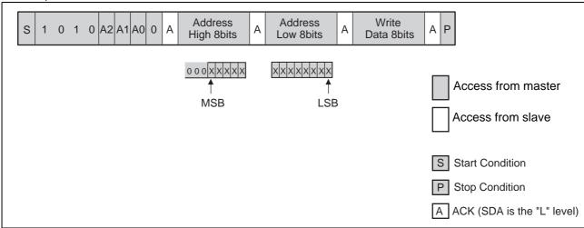
Note: In the MB85RC64A, input "000" as the upper 3 bits of the MSB.
