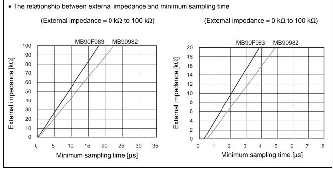
• If the sampling time cannot be sufficient, connect a capacitor of about 0.1  $\mu$ F to the analog input pin.
