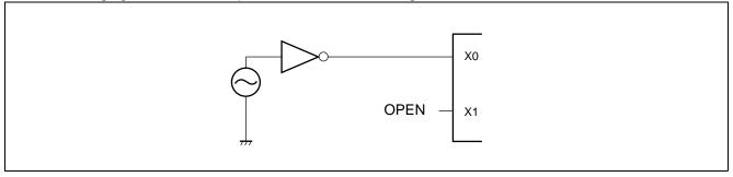
The following figure shows a sample use of external clock signals.
