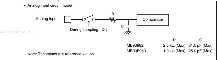
• To satisfy the A/D conversion precision standard, consider the relationship between the external impedance and minimum sampling time and either adjust the resistor value and operating frequency or decrease the external impedance so that the sampling time is longer than the minimum value.
