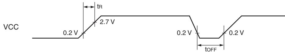
Note: Extreme variations in power supply voltage may trigger a power-on reset. When the power supply voltage is changed during operation, it is recommended that increases in voltage are smoothed out as shown in the following diagram. The PLL clock of the device should not be in use when varying the voltage. However, the PLL clock may continue to be used if the rate of the voltage drop is 1 V/s or less.
