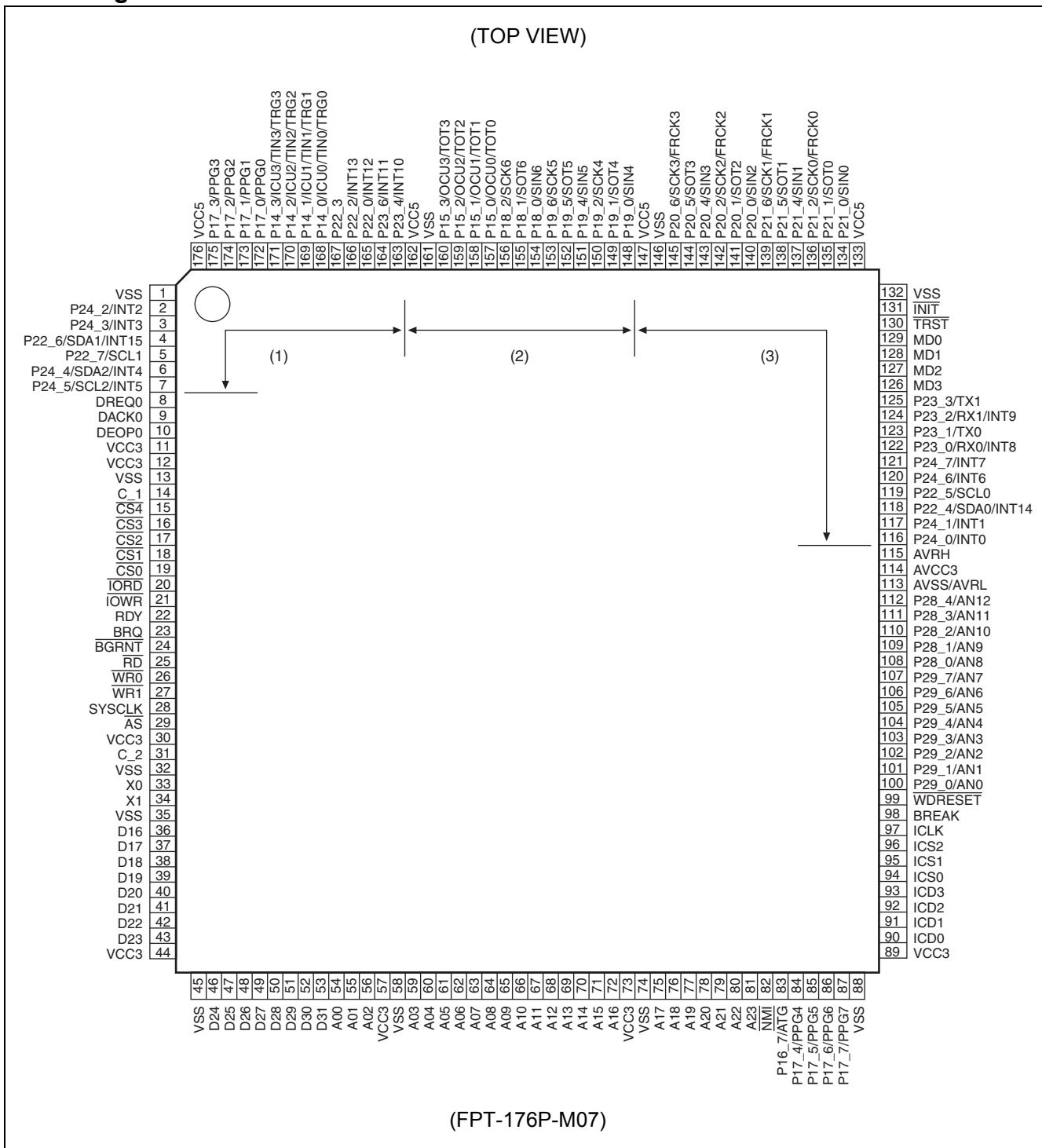
Note : (1) to (3) are 3.3 V/5 V pin supported pin, and can set 3.3 V and 5 V to the voltage in each block. I<sup>2</sup>C pin in (1) can be inputted at 5 V power supply. However, 3.3 V of the input threshold value is used as the standard value regardless of the power supply voltage. If 5 V is set in (1) or (2), also set 5 V to (3).
