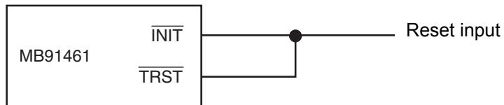
Since the reset pin (TRST) for development tool is the input pin supporting 3V/5V, it can be connected to INIT pin directly.
