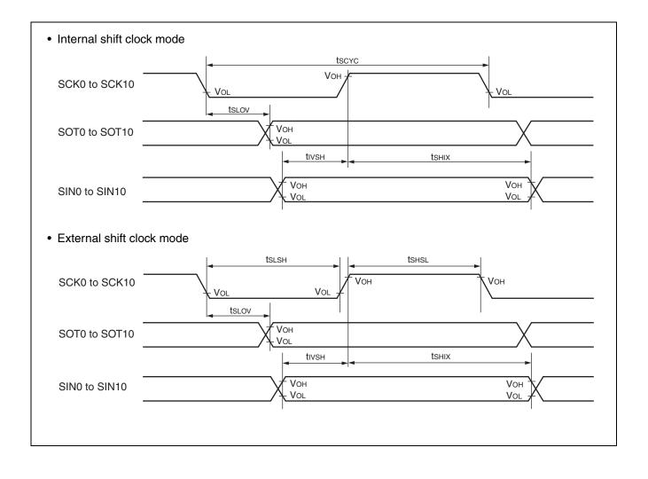
(5) Free-run timer clock, Reload timer event Input, up down counter Input, Input capture Input, Interrupt Input Timing
