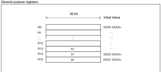
Registers R0 to R15 are general purpose registers. The registers are used as the accumulator and memory access pointers for CPU operations.
