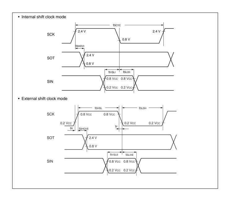
Sampling at the rising edge of sampling  $clock^{*1}$  and enabled serial clock delay\*<sup>2</sup> (ESCR register : SCES bit = 0, ECCR register : SCDE bit = 1)
