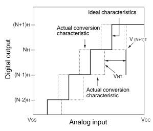
$$\frac{\text{Linearity error in}}{\text{digital output N}} = \frac{V_{\text{NT}} - \{1 \text{ LSB} \times \text{N} + \text{Vot}\}}{1 \text{ LSB}}$$
