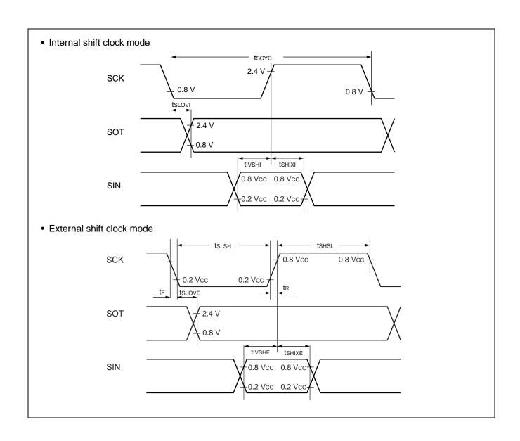
Sampling at the falling edge of sampling clock\*1 and prohibited serial clock delay\*2 (ESCR register : SCES bit = 1, ECCR register : SCDE bit = 0)
