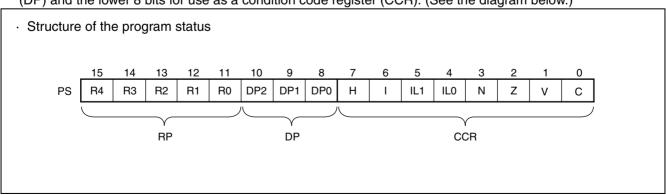
The RP indicates the address of the register bank currently being used. The relationship between the content of RP and the real address conforms to the conversion rule illustrated below:
