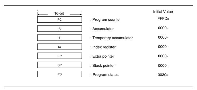
The PS can further be divided into higher 8 bits for use as a register bank pointer (RP) and a direct bank pointer (DP) and the lower 8 bits for use as a condition code register (CCR). (See the diagram below.)
