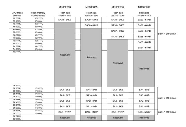
\*: Physical address area of SAS-512B is from DF:0000<sub>H</sub> to DF:01FF<sub>H</sub>. Others (from DF:0200<sub>H</sub> to DF:1FFF<sub>H</sub>) is mirror area of SAS-512B. Sector SAS contains the ROM configuration block RCBA at CPU address DF:0000<sub>H</sub> -DF:01FF<sub>H</sub>. SAS can not be used for E<sup>2</sup>PROM emulation.
