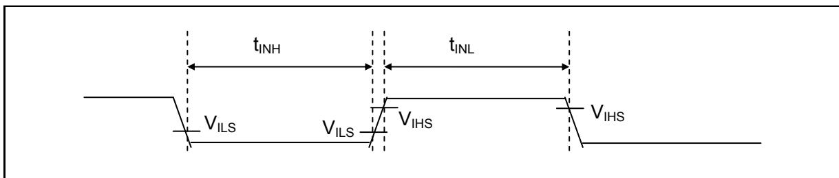
(10) I<sup>2</sup>C timing(V<sub>CC</sub> = AV<sub>CC</sub> = 2.7V to 5.5V, V<sub>SS</sub> = AV<sub>SS</sub> = 0V, T<sub>A</sub> = -40°C to +125°C)
