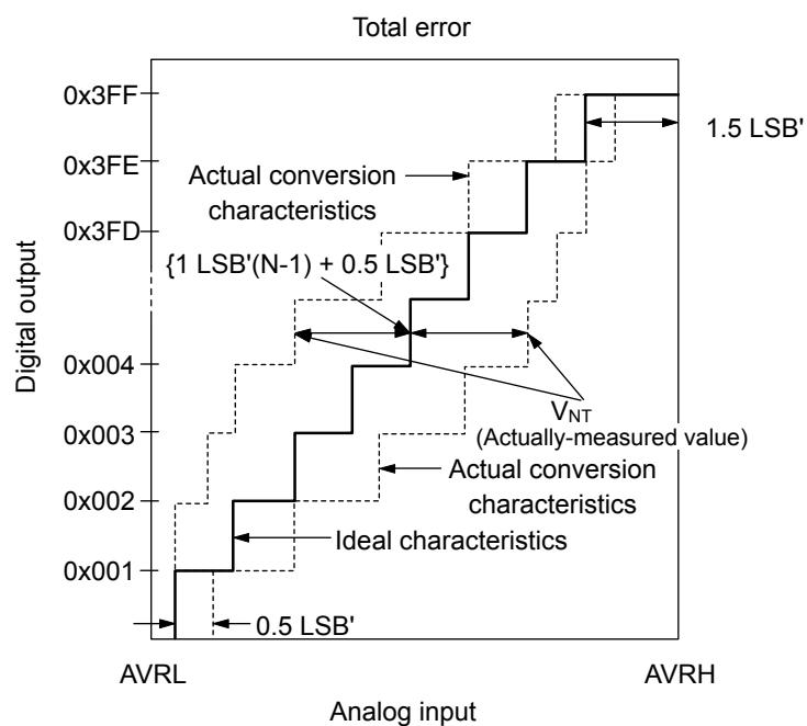
$$1\text{LSB}' \text{ (Ideal value)} = \frac{\text{AVRH} - \text{AVRL}}{1024} \text{ [V]}$$
