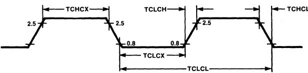
**AC Testing Input/Output and Float Waveforms**
