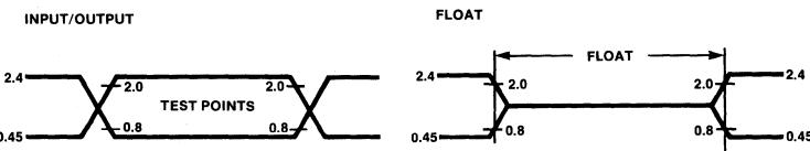
AC inputs during testing are driven at 2.4V for a logic "1" and 0.45V for a logic "0". Timing measurements are made at 2.0V for a logic "1" and 0.8V for a logic "0". For timing purposes, the float state is defined as the point at which a P0 pin sinks 3.2mA or sources 400µA at the voltage test levels.
