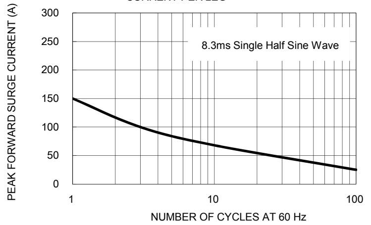
FIG. 2- MAXIMUM NON-REPETITIVE FORWARD SURGE CURRENT PER LEG
