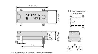
The metal case inside of the molding compound may be exposed on the top or bottom of this product. This purely cosmetic and does not have any effect on quality, reliability or electrical specs.
