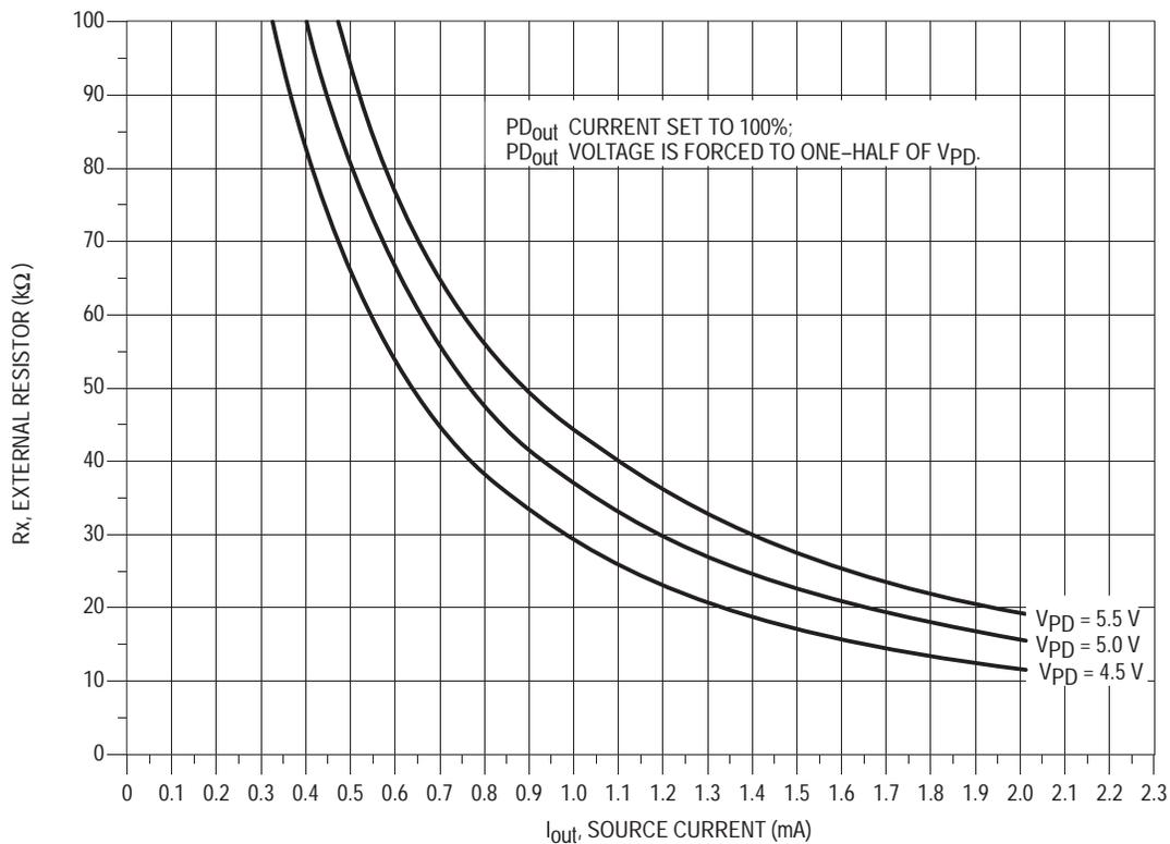
**Nominal MC145191 PD<sub>out</sub> Source Current vs Rx Resistance**
