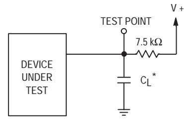
\*Includes all probe and fixture capacitance.
