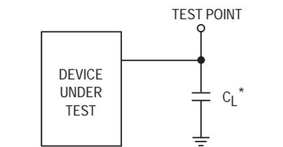
\*Includes all probe and fixture capacitance.
