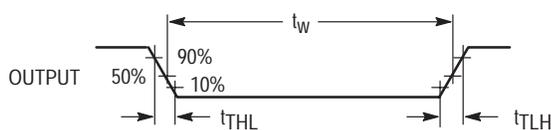
Figure 11. Switching Waveform
