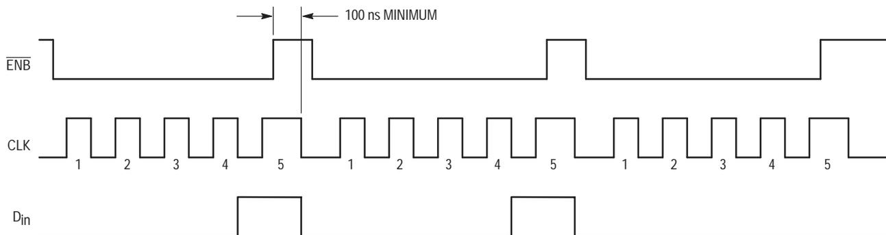
NOTE: It may not be convenient to control the  $\overline{\text{ENB}}$  or CLK pins during power up per the Pin Descriptions. If this is the case, the part may be initialized through the serial port as shown in the figure above. The sequence is similar to accessing the registers except that the CLK must remain high at least 100 ns after  $\overline{\text{ENB}}$  is brought high. Note that 3 groups of 5 bits are needed.
