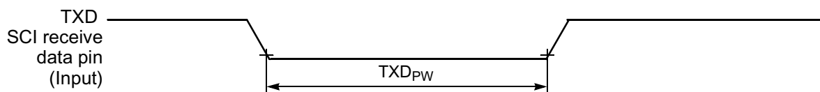
Figure 10-17 TXD Pulse Width
