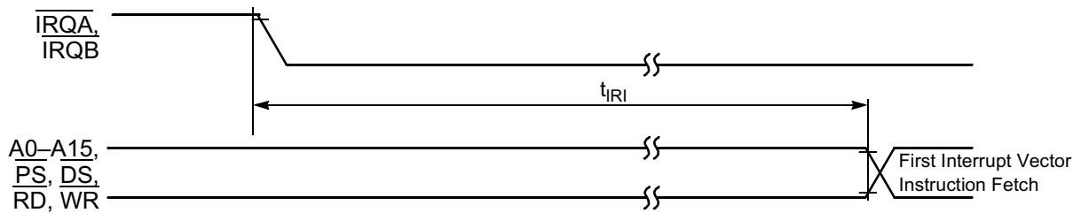
Figure 10-8 Interrupt from Wait State Timing
