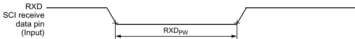
Figure 10-16 RXD Pulse Width
