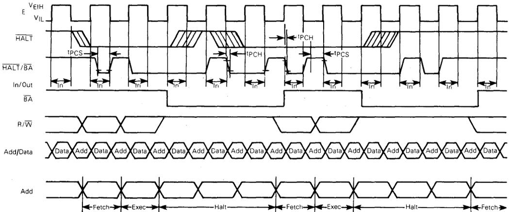
Note: Timing measurements are referenced to and from a low voltage of 0.8 volts and a high voltage of 2.0 volts, unless otherwise noted.
