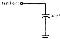
FIGURE 2 — TIMING TEST LOAD PORTS 2, 3, 4
