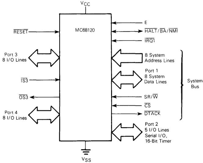
FIGURE 26 — EXPANDED NON-MULTIPLEXED MODE
