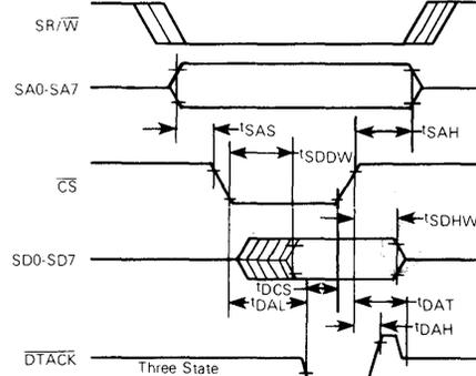
Note: Timing measurements are referenced to and from a low voltage of 0.8 volts and a high voltage of 2.0 volts, unless otherwise noted.
