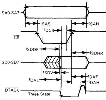
FIGURE 12 — ASYNCHRONOUS WRITE OF RAM
