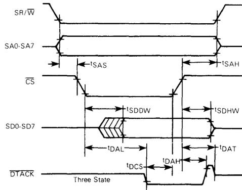
FIGURE 11 — ASYNCHRONOUS READ OF RAM
