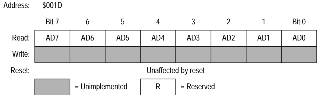
Figure 11-2. A/D Conversion Value Data Register (ADC)
