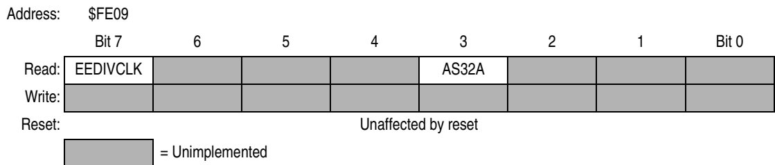
Figure 10-2. Mask Option Register 2 (MORB)
