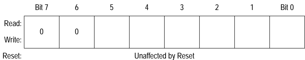
Figure 12-3. PWM Data Register (PWMDR)
