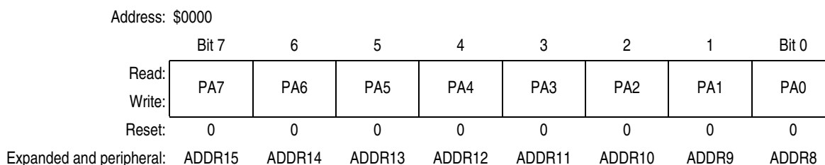
Figure 6-1. Port A Data Register (PORTA)
