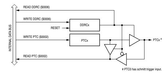
Figure 18-11. Port C I/O Circuit
