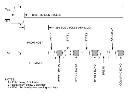
Figure 10-8. Monitor Mode Entry Timing
