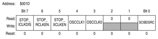
Figure 7-3. Configuration Register 2 (CONFIG2)
