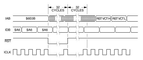
Figure 9-17. Wait Recovery from Internal Reset
