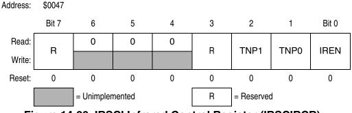
Figure 14-20. IRSCI Infrared Control Register (IRSCIRCR)
