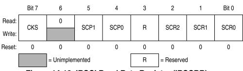
Figure 14-19. IRSCI Baud Rate Register (IRSCBR)
