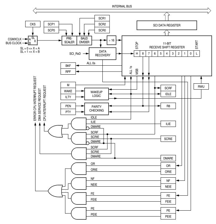
Figure 14-8. SCI Receiver Block Diagram
