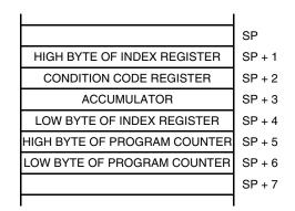
Figure 10-7. Stack Pointer at Monitor Mode Entry
