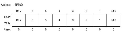
Figure 23-5. Break Address Register Low (BRKL)
