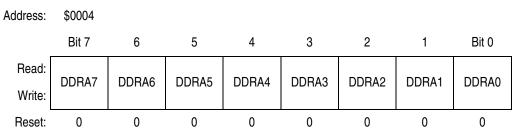
Figure 18-3. Data Direction Register A (DDRA)
