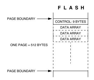
Figure 10-10. EE\_WRITE FLASH Memory Usage
