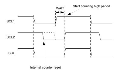
Figure 16-3. Clock Synchronization
