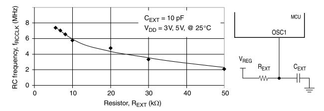
Figure 24-1. RC vs. Frequency
