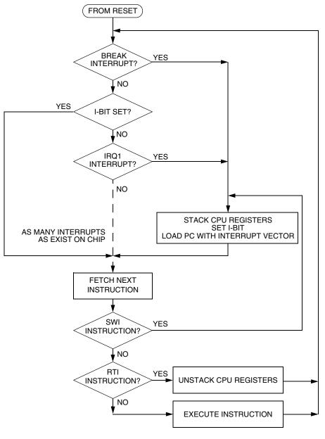
Figure 9-10. Interrupt Processing
