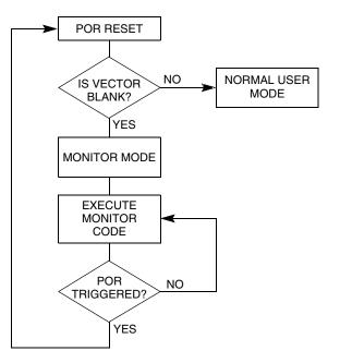
Figure 10-2. Low-Voltage Monitor Mode Entry Flowchart
