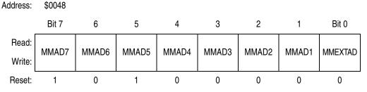
Figure 16-4. MMIIC Address Register (MMADR)
