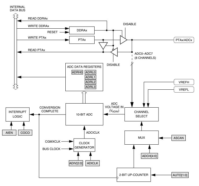
Figure 17-2. ADC Block Diagram
