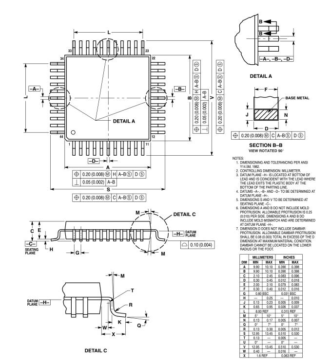
Figure 25-2. 44-Pin QFP (Case #824A)
