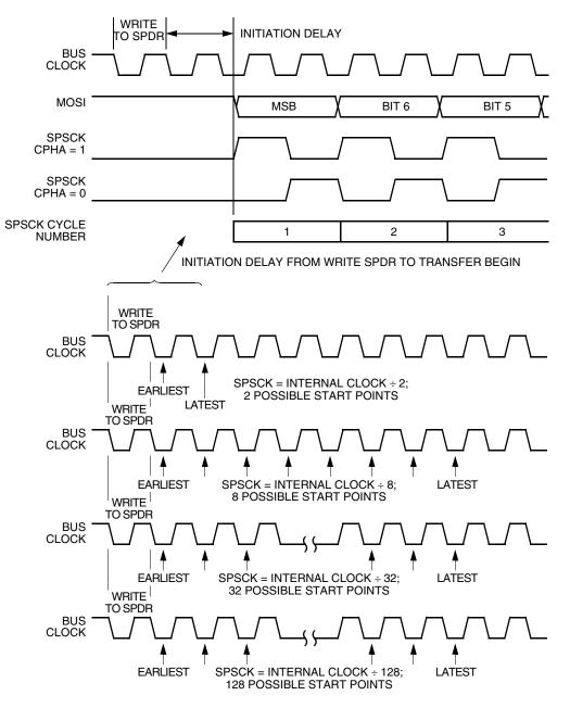
Figure 15-7. Transmission Start Delay (Master)
