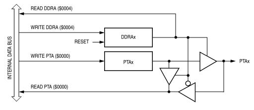
Figure 18-4. Port A I/O Circuit
