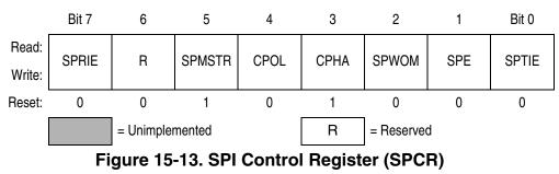
SPRIE — SPI Receiver Interrupt Enable Bit
