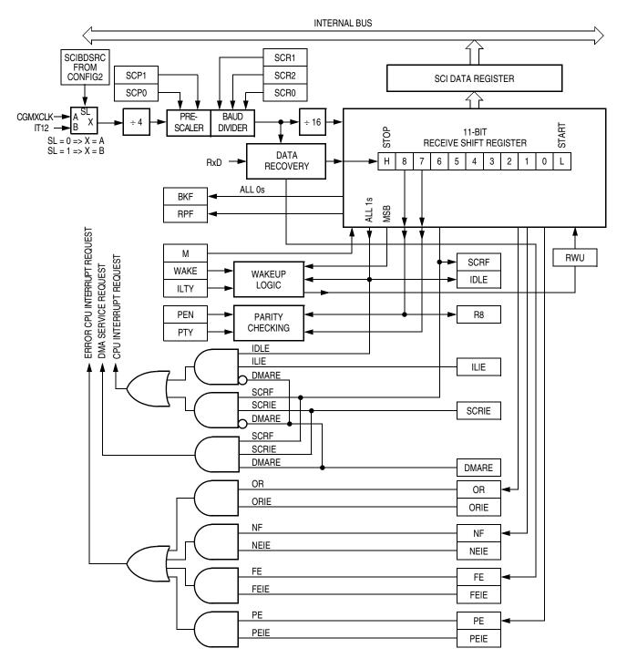
Figure 13-5. SCI Receiver Block Diagram
