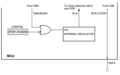
Figure 7-4. Internal Oscillator
