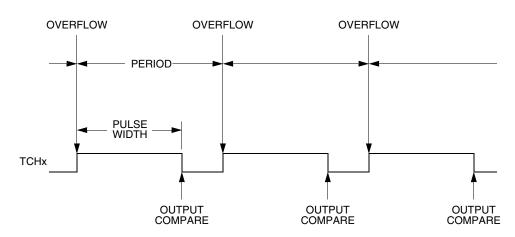
Figure 11-3. PWM Period and Pulse Width
