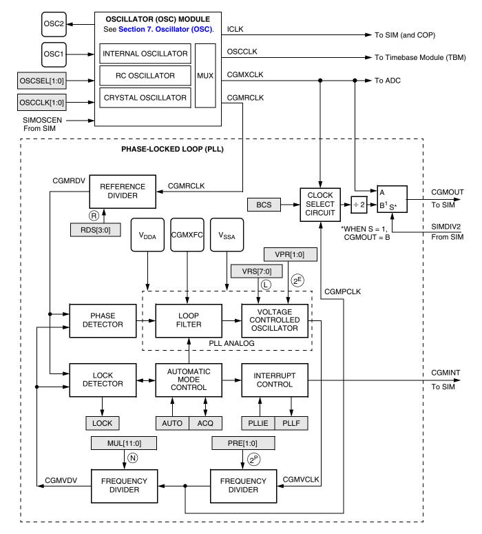
Figure 8-1. CGM Block Diagram
