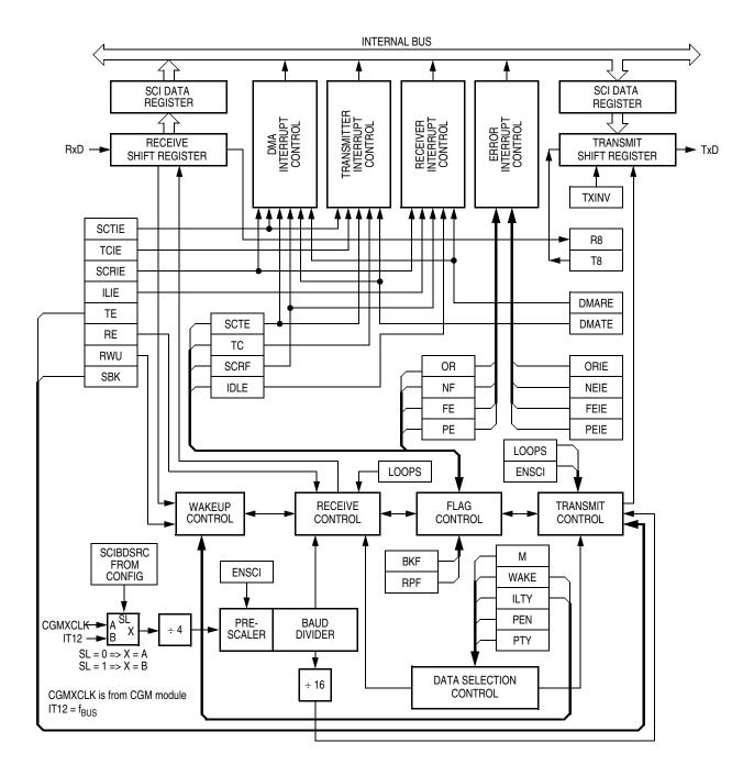
Figure 13-1. SCI Module Block Diagram
