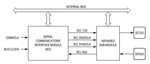
Figure 14-2. IRSCI Block Diagram
