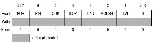
Figure 9-21. SIM Reset Status Register (SRSR)
