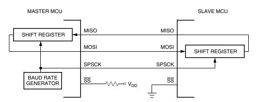
Figure 15-3. Full-Duplex Master-Slave Connections
