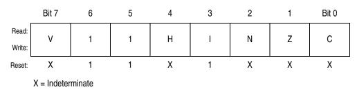
Figure 6-6. Condition Code Register (CCR)
