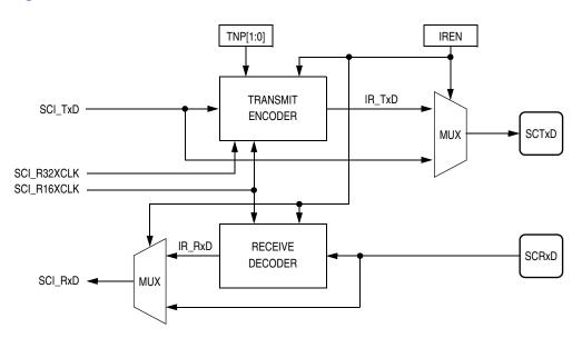
Figure 14-3 shows the structure of the infrared sub-module.
