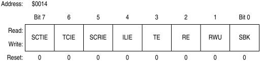
Figure 13-10. SCI Control Register 2 (SCC2)
