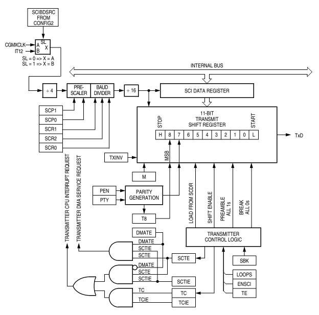
Figure 13-4. SCI Transmitter
