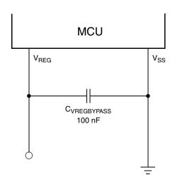
Figure 1-6. Regulator Power Supply Bypassing
