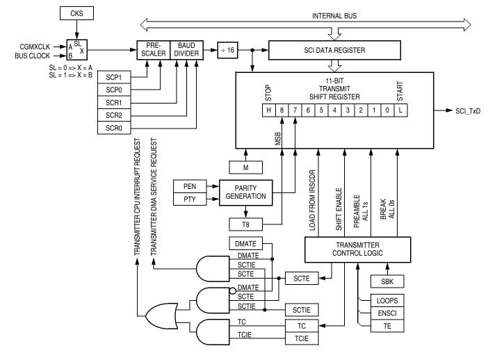
Figure 14-7. SCI Transmitter
