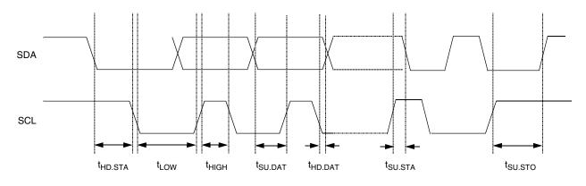
Figure 24-2. MMIIC Signal Timings
