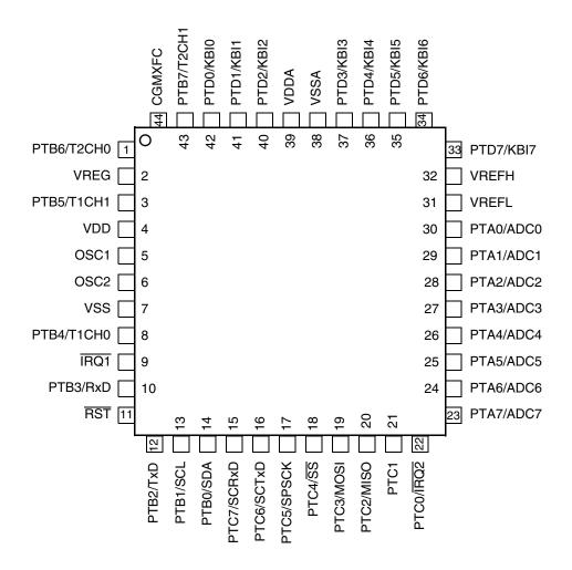
Figure 1-3. 44-Pin QFP Pin Assignments
