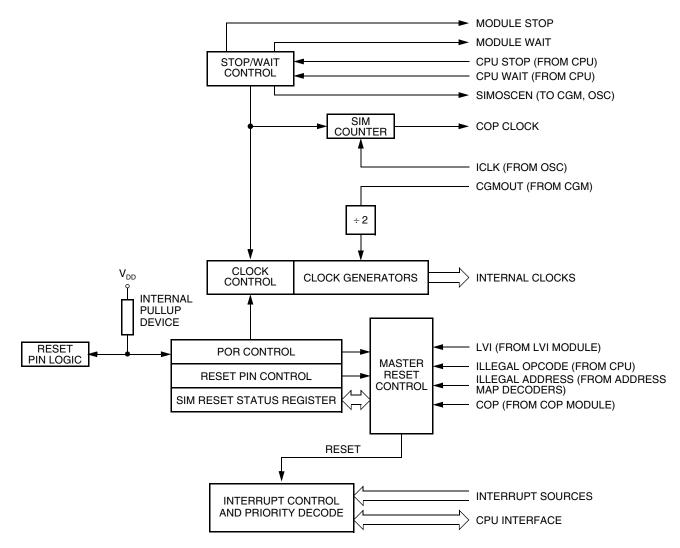
Figure 9-1. SIM Block Diagram
