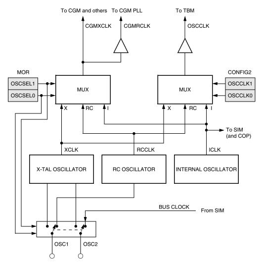
Figure 7-1. Oscillator Module Block Diagram
