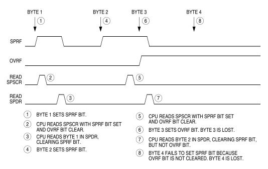
Figure 15-9. Missed Read of Overflow Condition
