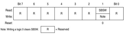
Figure 9-20. SIM Break Status Register (SBSR)
