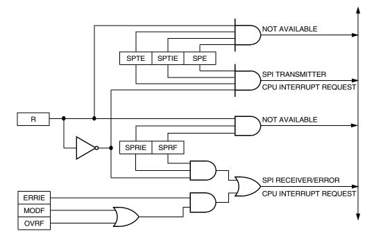
Figure 15-11. SPI Interrupt Request Generation
