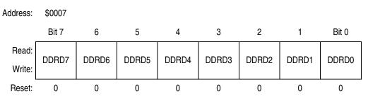
Figure 18-13. Data Direction Register D (DDRD)
