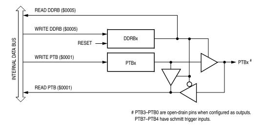
Figure 18-8. Port B I/O Circuit
