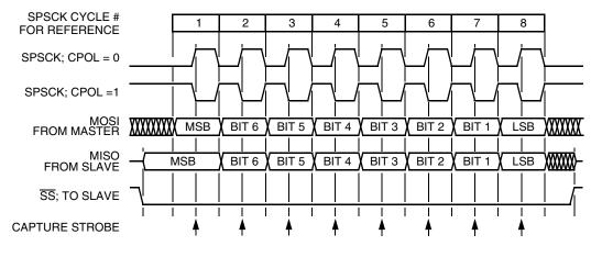
Figure 15-4. Transmission Format (CPHA = 0)
