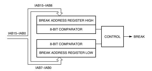
Figure 23-1. Break Module Block Diagram
