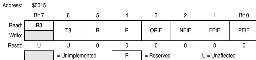
Figure 18-13. SCI Control Register 3 (SCC3)
