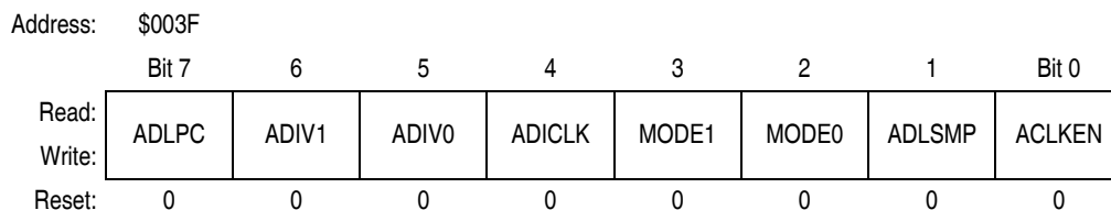
Figure 3-7. ADC10 Clock Register (ADCLK)
