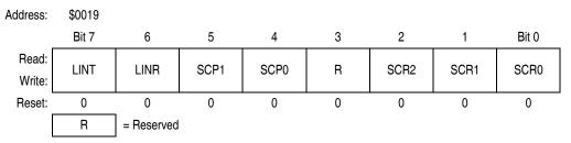
Figure 14-17. ESCI Baud Rate Register (SCBR)
