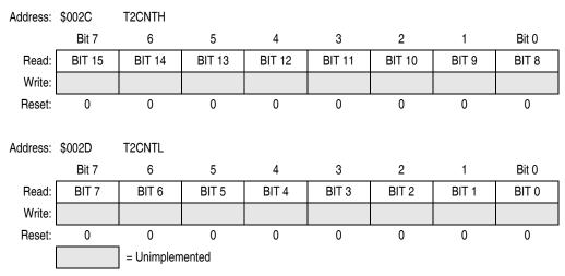
Figure 19-6. TIM2 Counter Registers (T2CNTH and T2CNTL)
