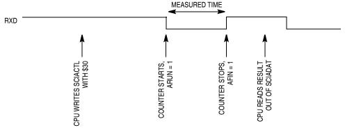
Figure 14-23. Bit Time Measurement with ACLK = 1, Scenario B
