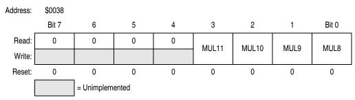
Figure 4-6. PLL Multiplier Select Register High (PMSH)
