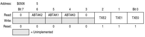
Figure 12-22. Transmitter Flag Register (CTFLG)
