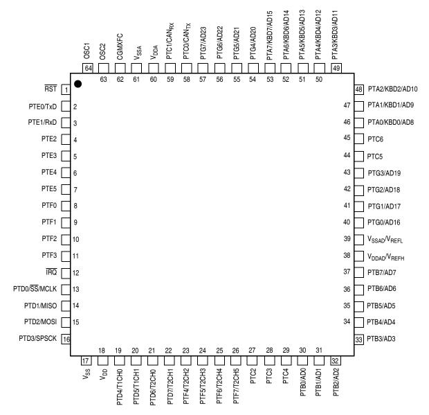
Figure 1-4. 64-Pin QFP Pin Assignments
