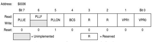
Figure 4-4. PLL Control Register (PCTL)
