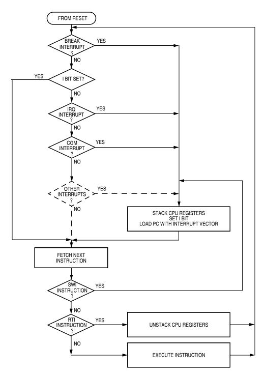
Figure 15-10. Interrupt Processing
