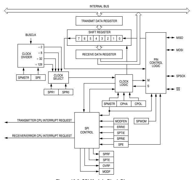
Figure 16-2. SPI Module Block Diagram
