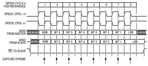
Figure 16-7. Transmission Format (CPHA = 1)
