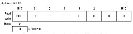
Figure 20-8. Break Flag Control Register (BFCR)
