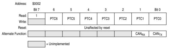
Figure 13-9. Port C Data Register (PTC)
