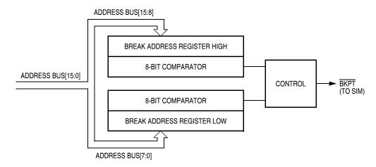
Figure 20-2. Break Module Block Diagram
