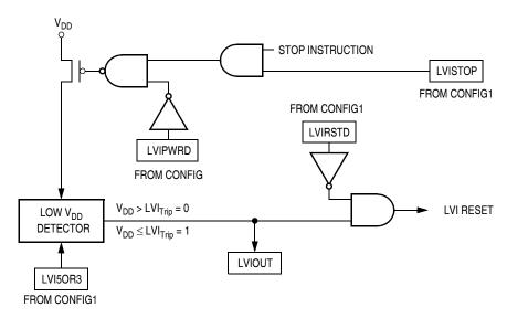
Figure 11-1. LVI Module Block Diagram
