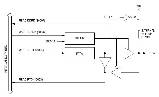
Figure 13-15. Port D I/O Circuit
