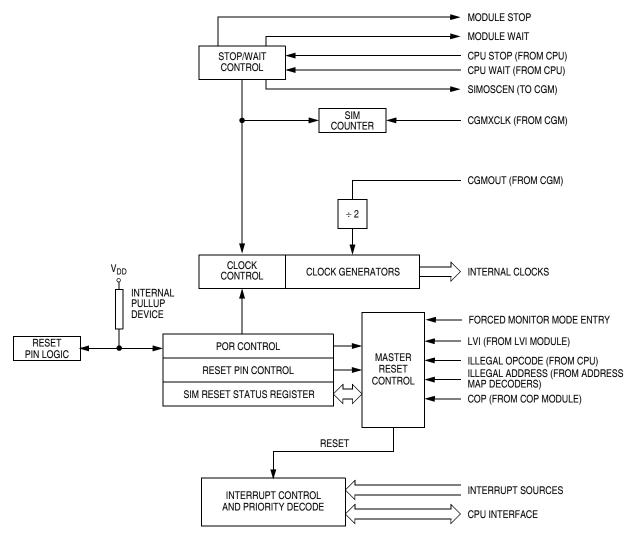
Figure 15-1. SIM Block Diagram
