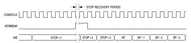
Figure 15-20. Stop Mode Recovery from Interrupt
