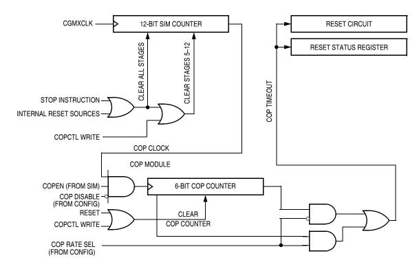
Figure 6-1. COP Block Diagram
