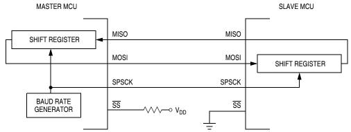
Figure 16-4. Full-Duplex Master-Slave Connections
