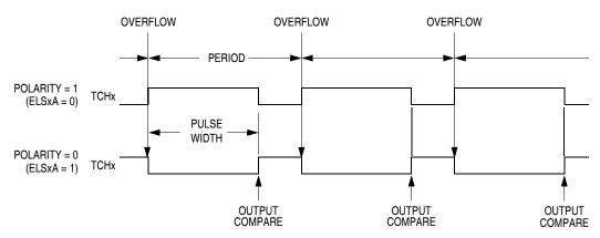
Figure 18-4. PWM Period and Pulse Width
