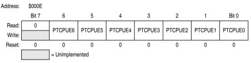
Figure 13-12. Port C Input Pullup Enable Register (PTCPUE)
