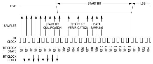
Figure 14-7. Receiver Data Sampling
