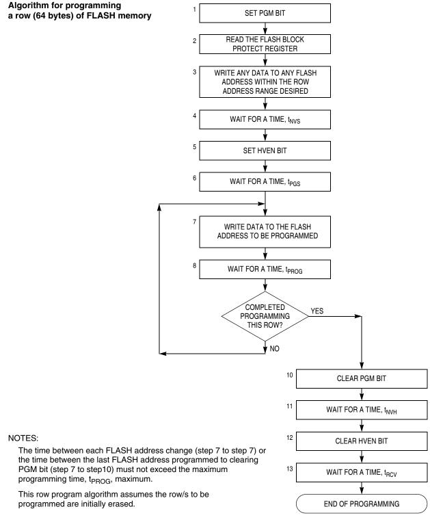
Figure 2-10. FLASH-2 Programming Algorithm Flowchart
