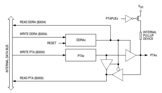
Figure 13-4. Port A I/O Circuit
