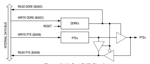
Figure 13-19. Port E I/O Circuit Table 13-6. Port E Pin Functions
