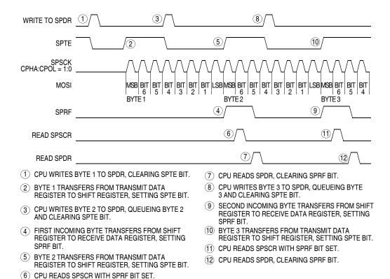
Figure 16-9. SPRF/SPTE CPU Interrupt Timing
