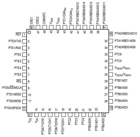
Figure 1-3. 48-Pin LQFP Pin Assignments
