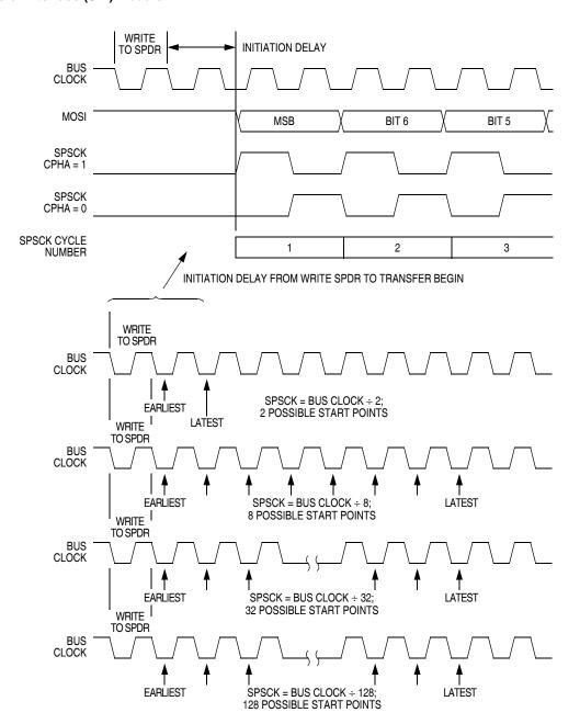
Figure 16-8. Transmission Start Delay (Master)
