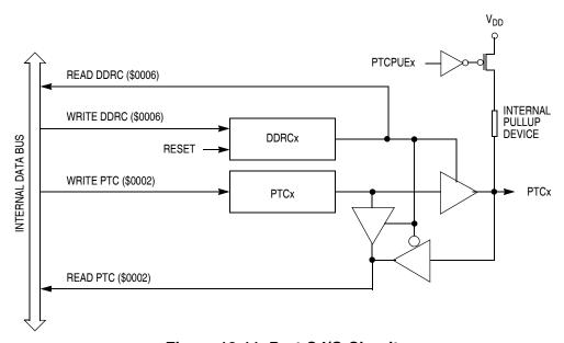
Figure 13-11. Port C I/O Circuit
