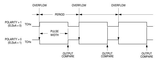
Figure 19-4. PWM Period and Pulse Width
