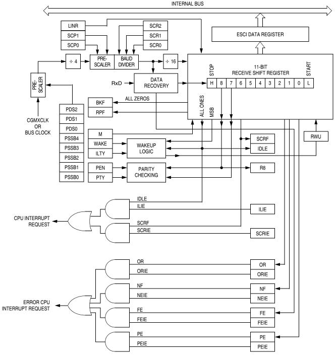
Figure 14-6. ESCI Receiver Block Diagram
