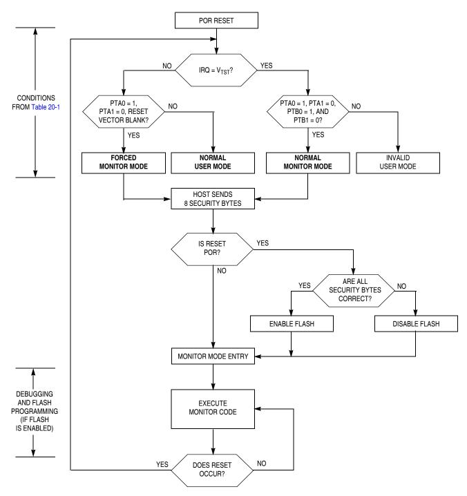
Figure 20-9. Simplified Monitor Mode Entry Flowchart
