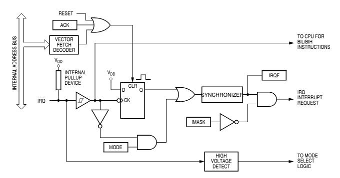
Figure 8-1. IRQ Module Block Diagram
