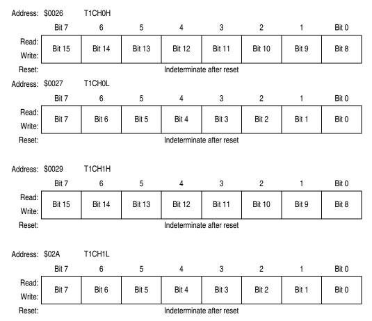
Figure 18-10. TIM1 Channel Registers (T1CH0H/L:T1CH1H/L)
