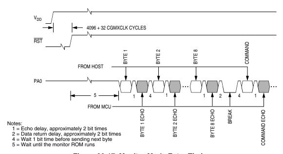
Figure 20-17. Monitor Mode Entry Timing
