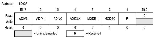
Figure 3-9. ADC Clock Register (ADCLK)
