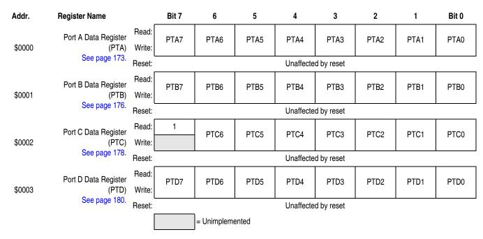
Figure 13-1. I/O Port Register Summary (Sheet 1 of 3)
