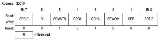
Figure 16-14. SPI Control Register (SPCR)
