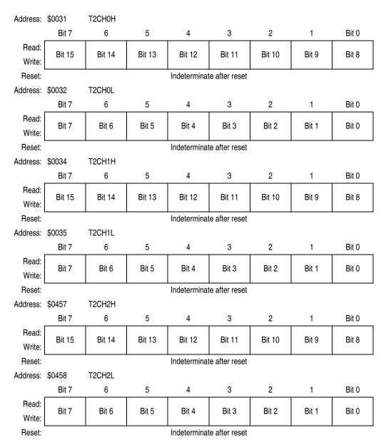
Figure 19-10. TIM2 Channel Registers (T2CH0H/L:T2CH5H/L)
