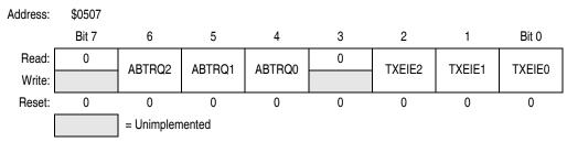
Figure 12-23. Transmitter Control Register (CTCR)
