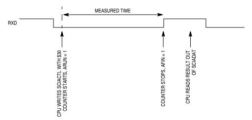
Figure 14-22. Bit Time Measurement with ACLK = 1, Scenario A
