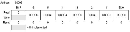
Figure 13-10. Data Direction Register C (DDRC)
