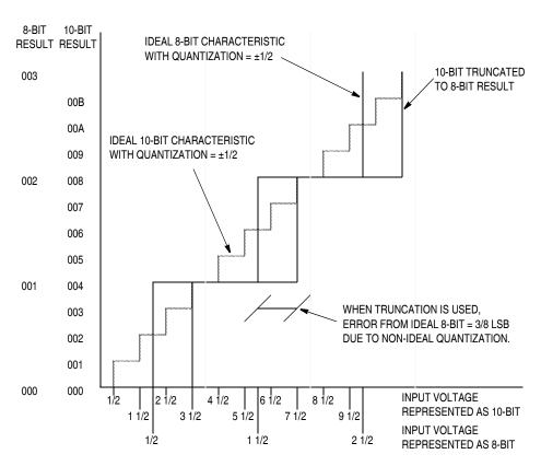
Figure 3-3. Bit Truncation Mode Error
