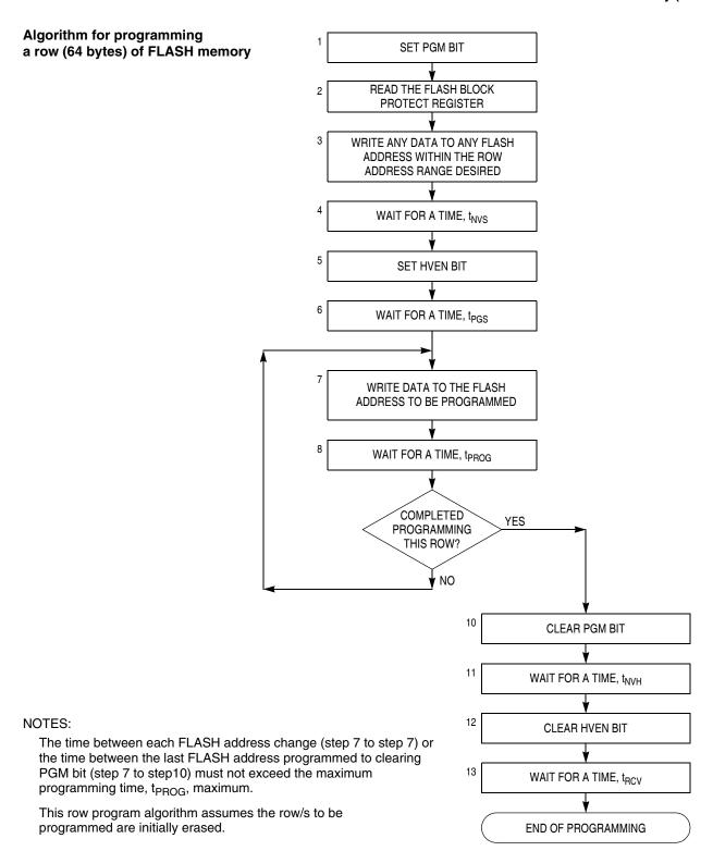
Figure 2-6. FLASH-1 Programming Algorithm Flowchart
