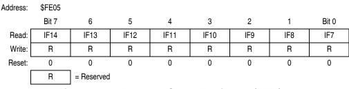
Figure 15-13. Interrupt Status Register 2 (INT2)
