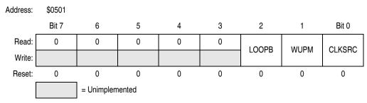
Figure 12-17. Module Control Register (CMCR1)
