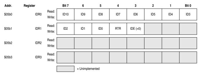
Figure 12-13. Standard Identifier Mapping
