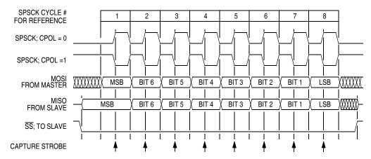
Figure 16-5. Transmission Format (CPHA = 0)
