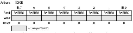
Figure 12-25. Receiver Error Counter (CRXERR)
