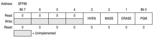
Figure 2-3. FLASH-1 Control Register (FL1CR)
