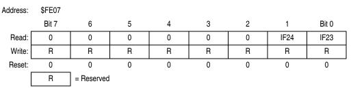
Figure 15-15. Interrupt Status Register 4 (INT4)
