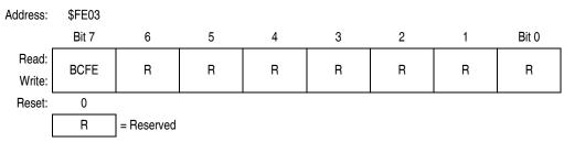
Figure 15-23. Break Flag Control Register (BFCR)
