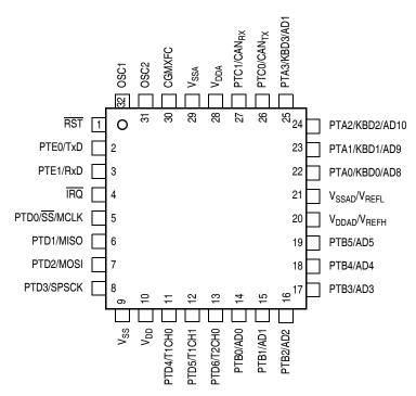
Figure 1-2. 32-Pin LQFP Pin Assignments
