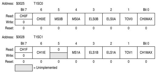
Figure 18-8. TIM1 Channel Status and Control Registers (T1SC0:T1SC1)
