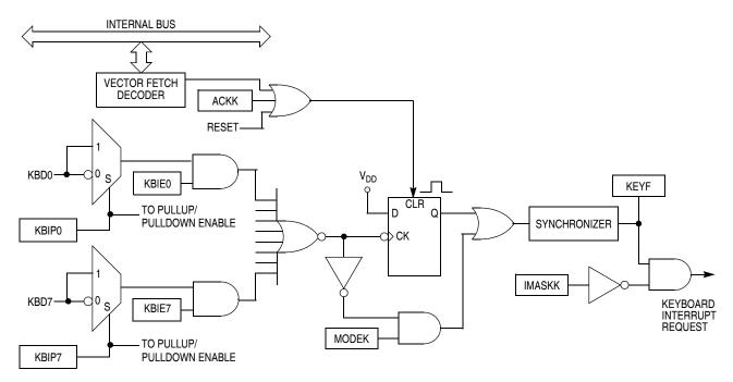
Figure 9-2. Keyboard Module Block Diagram
