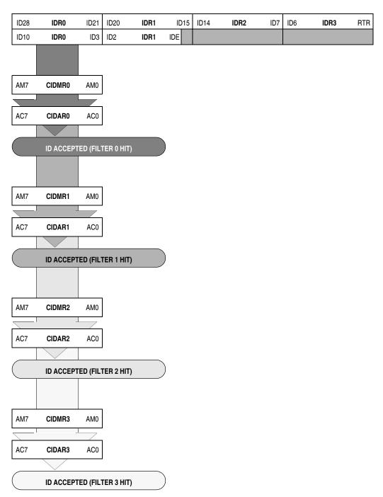
Figure 12-6. Quadruple 8-Bit Maskable Acceptance Filters
