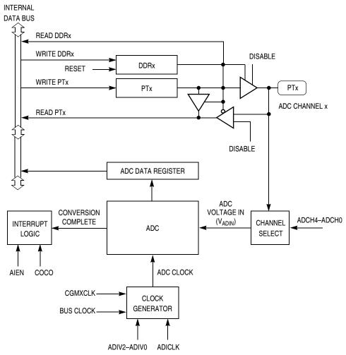
Figure 3-2. ADC Block Diagram
