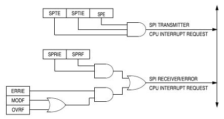
Figure 16-12. SPI Interrupt Request Generation
