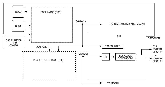
Figure 15-3. System Clock Signals
