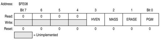
Figure 2-7. FLASH-2 Control Register (FL2CR)
