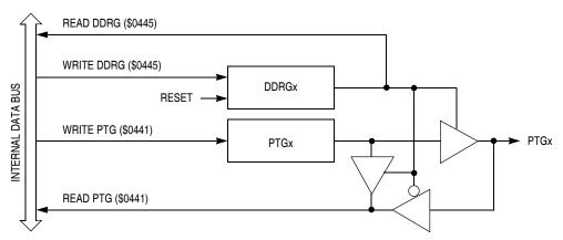
Figure 13-25. Port G I/O Circuit
