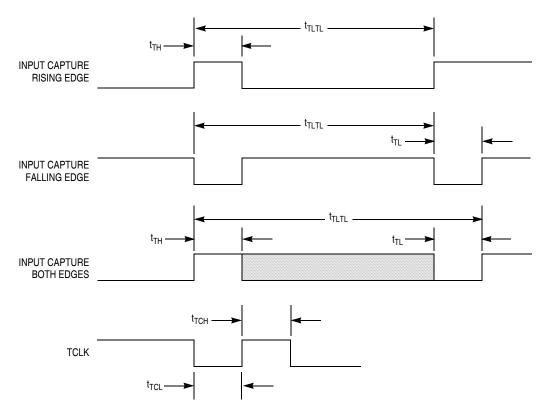
Figure 21-4. Timer Input Timing
