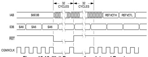
Figure 15-18. Wait Recovery from Internal Reset
