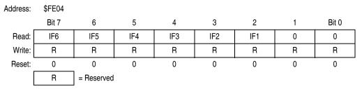
Figure 15-12. Interrupt Status Register 1 (INT1)
