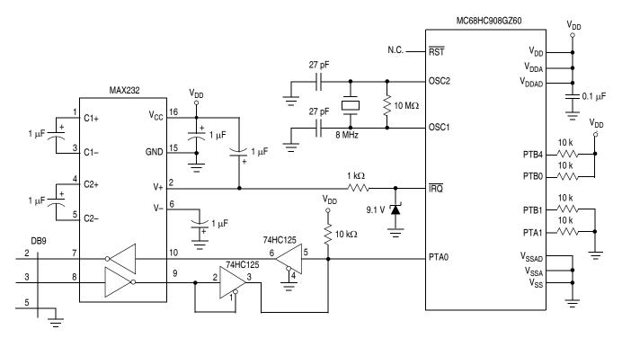
Figure 20-10. Normal Monitor Mode Circuit
