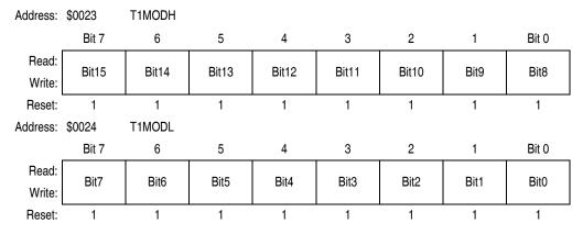
Figure 18-7. TIM1 Counter Modulo Registers (T1MODH:T1MODL)
