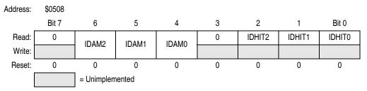
Figure 12-24. Identifier Acceptance Control Register (CIDAC)
