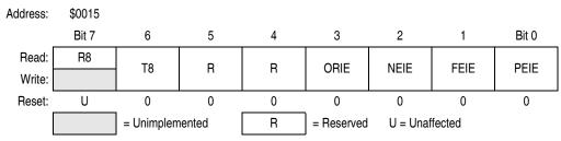
Figure 14-12. ESCI Control Register 3 (SCC3)
