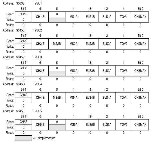
Figure 19-8. TIM2 Channel Status and Control Registers (T2SC0:T2SC5) (Continued)
