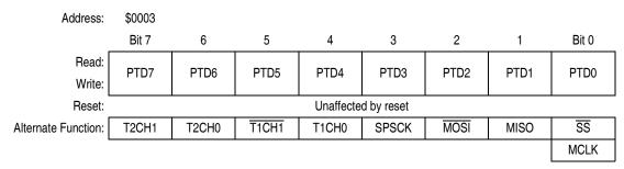
Figure 13-13. Port D Data Register (PTD)
