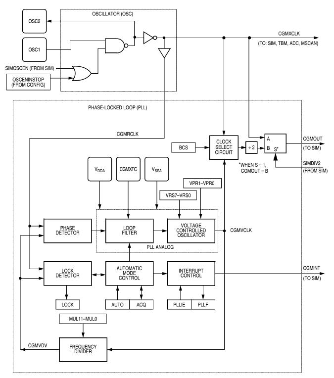
Figure 4-1. CGM Block Diagram
