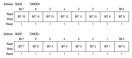
Figure 19-7. TIM2 Counter Modulo Registers (T2MODH and T2MODL)
