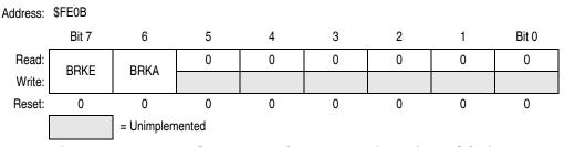
Figure 20-4. Break Status and Control Register (BRKSCR)
