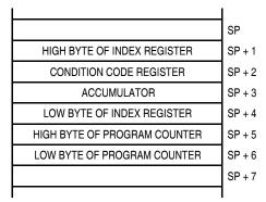
Figure 20-16. Stack Pointer at Monitor Mode Entry
