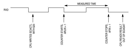
Figure 14-21. Bit Time Measurement with ACLK = 0
