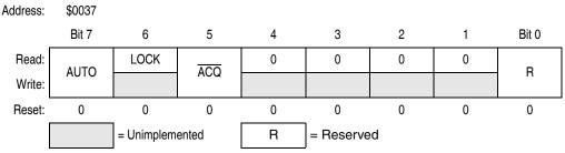
Figure 4-5. PLL Bandwidth Control Register (PBWC)
