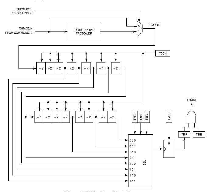
Figure 17-1. Timebase Block Diagram
