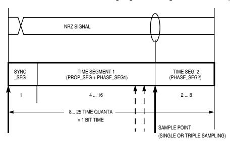
Figure 12-9. Segments Within the Bit Time
