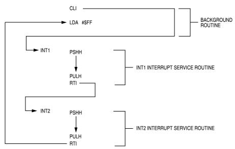
Figure 15-11. Interrupt Recognition Example
