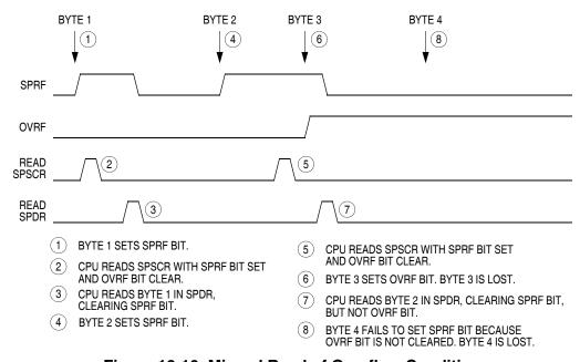
Figure 16-10. Missed Read of Overflow Condition
