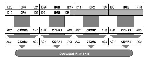
Figure 12-4. Single 32-Bit Maskable Identifier Acceptance Filter
