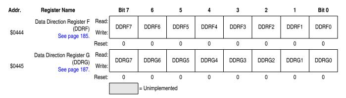
Figure 13-1. I/O Port Register Summary (Sheet 3 of 3)
