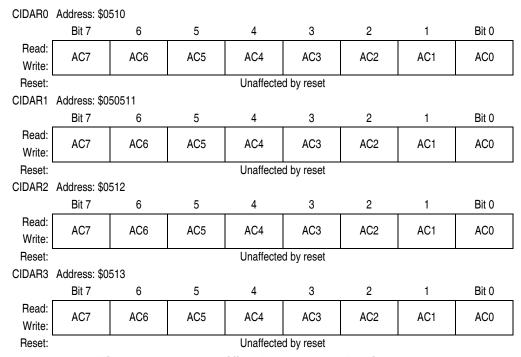
Figure 12-27. Identifier Acceptance Registers (CIDAR0–CIDAR3)
