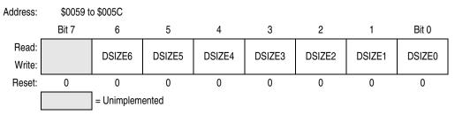
Figure 11-8. USB Endpoint 1-4 Data Size Register
