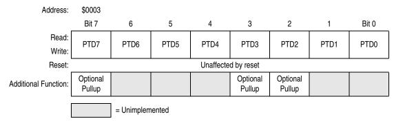
Figure 13-11. Port D Data Register (PTD)
