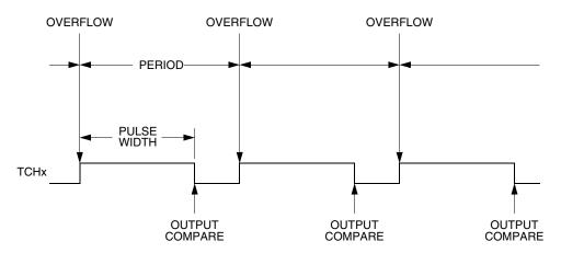
Figure 8-3. PWM Period and Pulse Width
