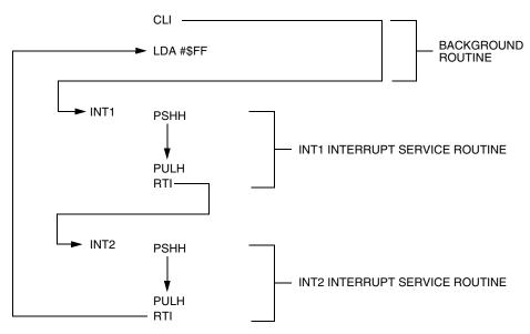
Figure 6-11. Interrupt Recognition Example
