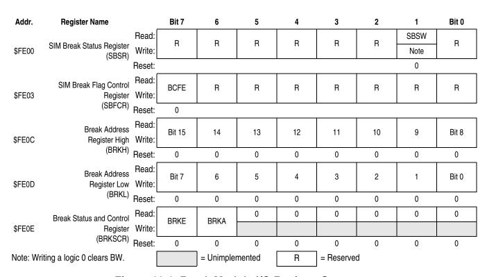
Figure 18-1. Break Module I/O Register Summary
