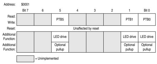
Figure 13-5. Port B Data Register (PTB)
