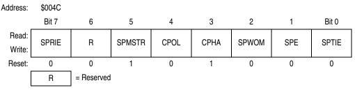
Figure 10-13. SPI Control Register (SPCR)
