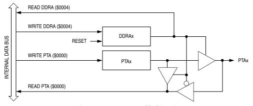
Figure 13-4. Port A I/O Circuit
