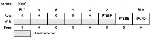
Figure 14-4. IRQ Option Control Register (IOCR)
