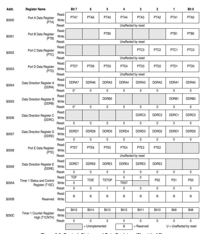
Figure 2-2. Control, Status, and Data Registers (Sheet 1 of 7)
