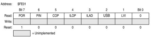
Figure 6-21. SIM Reset Status Register (SRSR)
