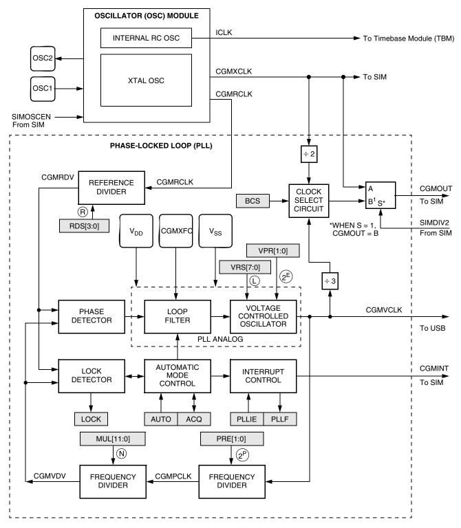
Figure 5-1. CGM Block Diagram
