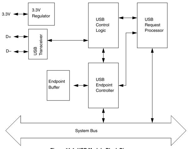
Figure 11-1. USB Module Block Diagram
