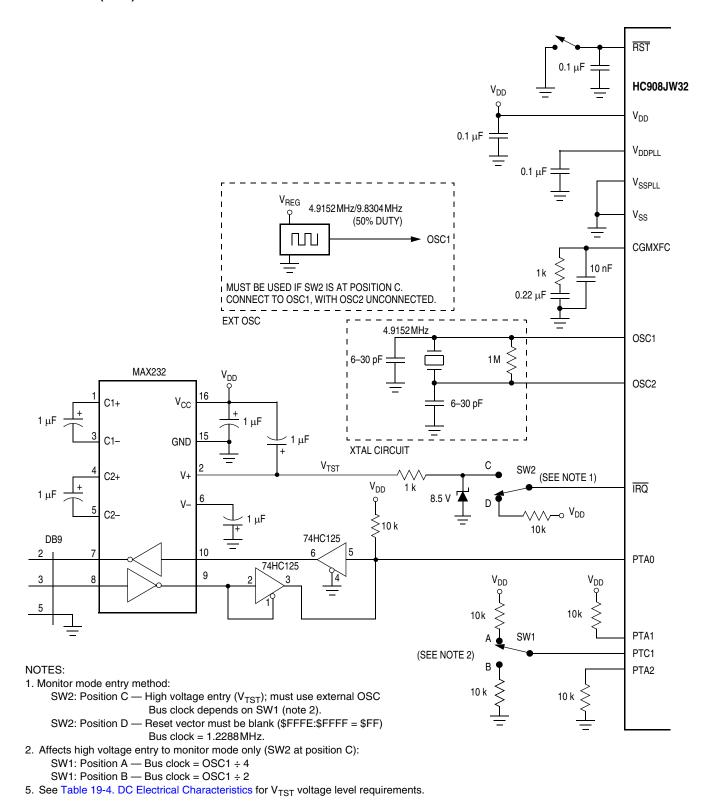
Figure 7-1. Monitor Mode Circuit
