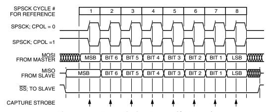
Figure 10-4. Transmission Format (CPHA = 0)
