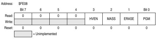
Figure 2-3. FLASH Control Register (FLCR)
