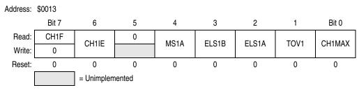
Figure 8-10. TIM Channel 1 Status and Control Register (TSC1)
