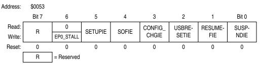
Figure 11-5. USB Status Interrupt Mask Register
