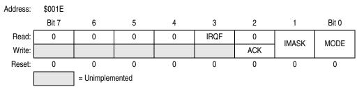
Figure 14-3. IRQ Status and Control Register (ISCR)
