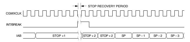
Figure 6-19. Stop Mode Recovery from Interrupt or Break
