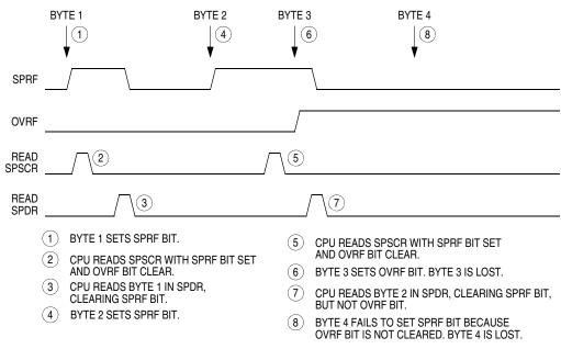
Figure 10-9. Missed Read of Overflow Condition
