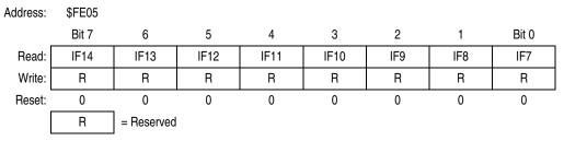
Figure 6-13. Interrupt Status Register 2 (INT2)
