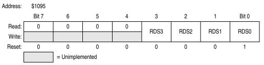
Figure 5-9. PLL Reference Divider Select Register (PMDS)
