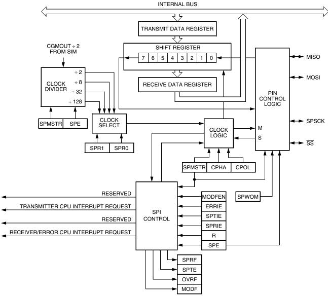
Figure 10-2. SPI Module Block Diagram
