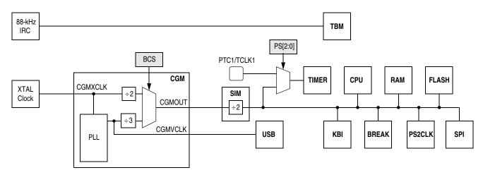
Figure 1-3. Clock Tree Diagram
