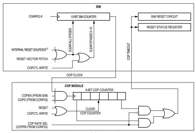
Figure 16-1. COP Block Diagram
