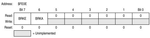
Figure 18-3. Break Status and Control Register (BRKSCR)
