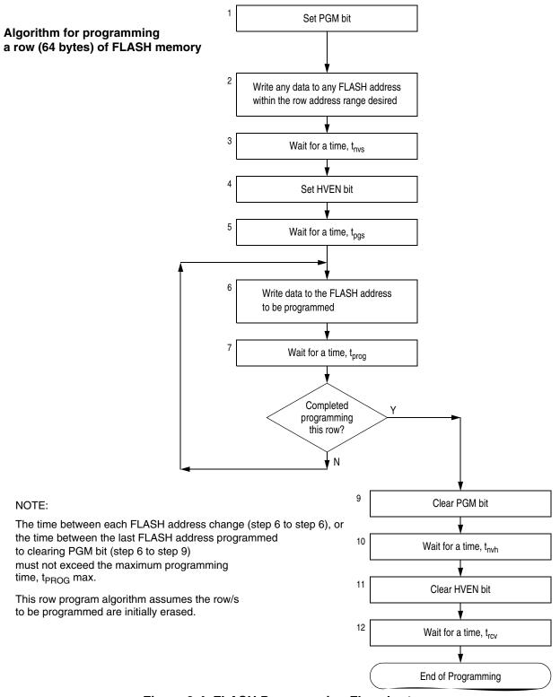
Figure 2-4. FLASH Programming Flowchart
