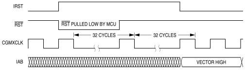
Figure 6-5. Internal Reset Timing
