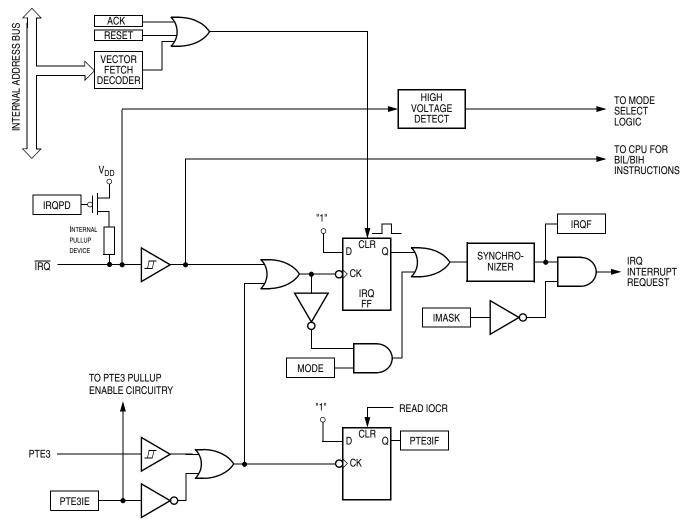
Figure 14-1. IRQ Module Block Diagram
