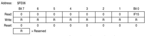
Figure 6-14. Interrupt Status Register 3 (INT3)
