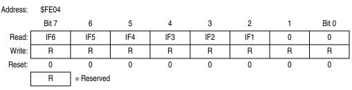
Figure 6-12. Interrupt Status Register 1 (INT1)
