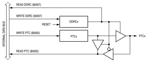
Figure 13-10. Port C I/O Circuit
