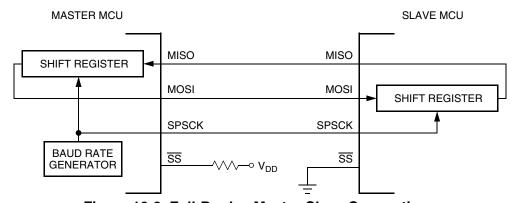
Figure 10-3. Full-Duplex Master-Slave Connections
