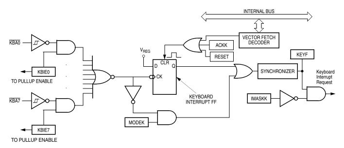
Figure 15-2. Keyboard Module Block Diagram
