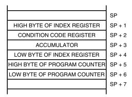
Figure 7-6. Stack Pointer at Monitor Mode Entry
