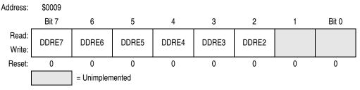
Figure 13-15. Data Direction Register E (DDRE)
