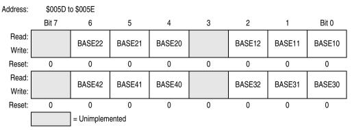
Figure 11-9. USB Endpoint 1-4 Data Pointer Register
