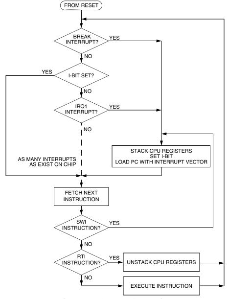
Figure 6-10. Interrupt Processing
