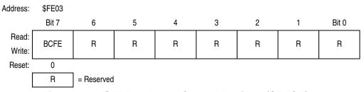
Figure 18-7. SIM Break Flag Control Register (SBFCR)
