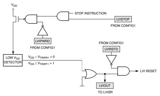
Figure 17-2. LVI Module Block Diagram
