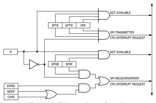
Figure 10-11. SPI Interrupt Request Generation
