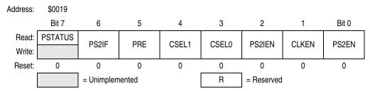
Figure 12-3. PS2 Clock Generator Control and Status Registers (PS2CSR)
