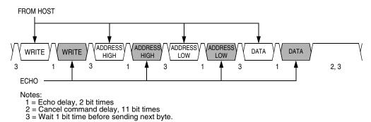
Figure 7-5. Write Transaction
