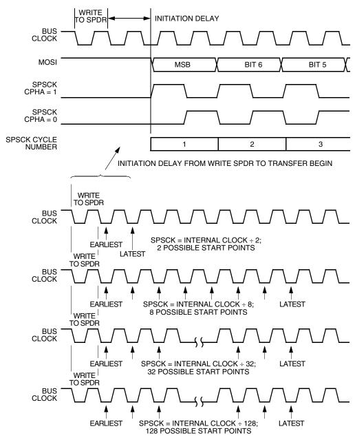
Figure 10-7. Transmission Start Delay (Master)
