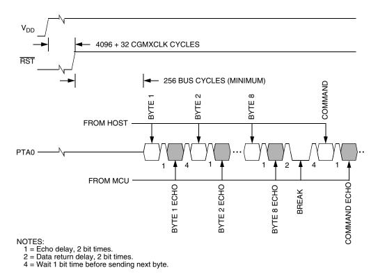
Figure 7-7. Monitor Mode Entry Timing
