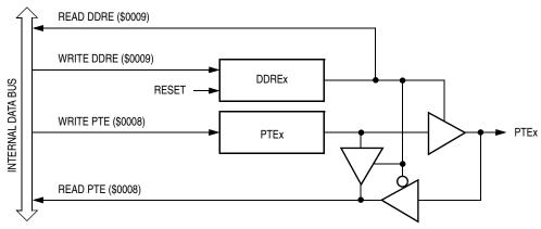
Figure 13-16. Port E I/O Circuit
