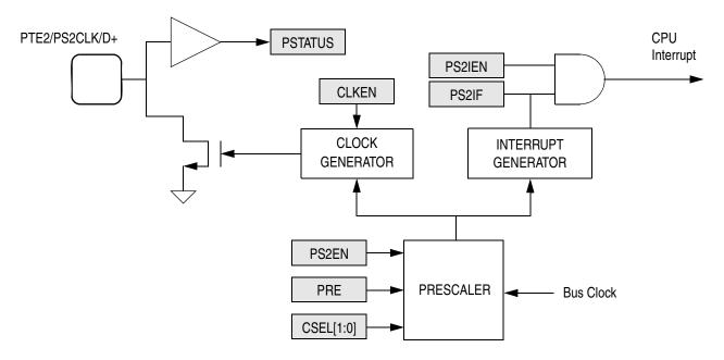
Figure 12-1. PS2 Clock Generator Block Diagram
