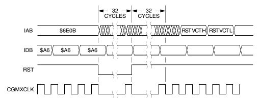
Figure 6-17. Wait Recovery from Internal Reset
