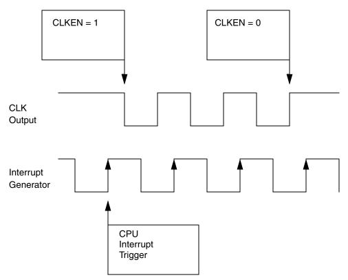
Figure 12-2. Clock Generator Output Waveform.
