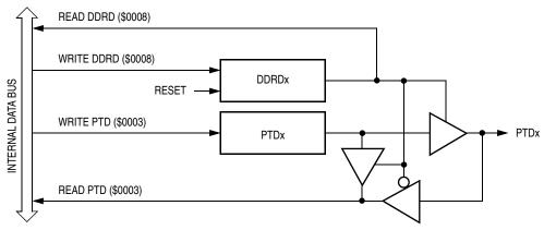
Figure 13-13. Port D I/O Circuit
