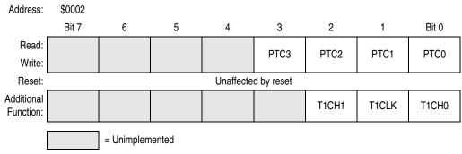
Figure 13-8. Port C Data Register (PTC)
