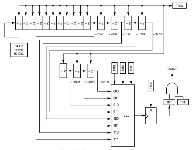
Figure 9-1. Timebase Block Diagram
