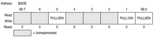
Figure 13-17. Pullup Control Register (PULLCR)
