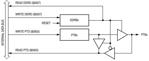
Figure 13-7. Port B I/O Circuit
