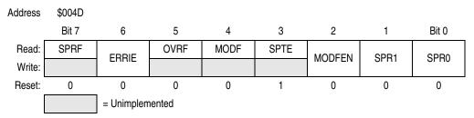
Figure 10-14. SPI Status and Control Register (SPSCR)
