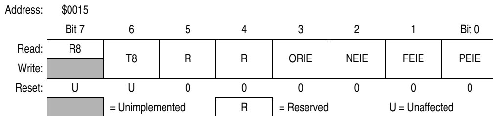
Figure 12-12. SCI Control Register 3 (SCC3)
