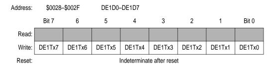
Figure 14-21. USB Embedded Device Endpoint 1/2 Data Registers (DE1D0-DE1D7)
