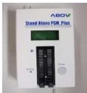
Figure 1-2 Stand Alone PGM_plus (Single Writer & ISP)
